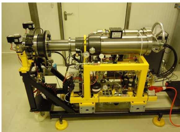
Fig. 3. Rapid compression expansion machine (RCEM) with a highly flexible optical access
