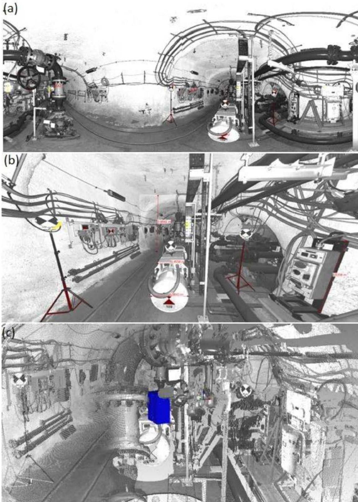
**Figure 4:** (a) Terrestrial laser scan (point cloud) in the engine room, (b) part of corresponding bubble view, and (c) corresponding scan in the form of XYZ coordinates.
