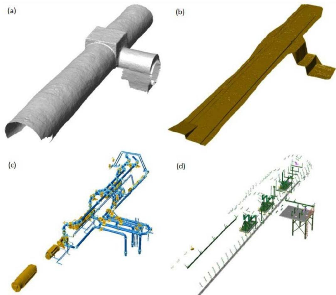
**Figure 6:** Classification or object recognition from the point cloud in 3D modelling process: (a) mine roadway walls, (b) ground surface, (c) pumps and pipelines, and (d) other features.
