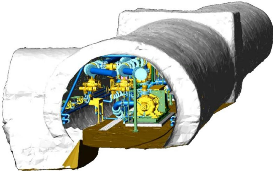
**Figure 7:** Complete 3D model of pumping station engine room.
