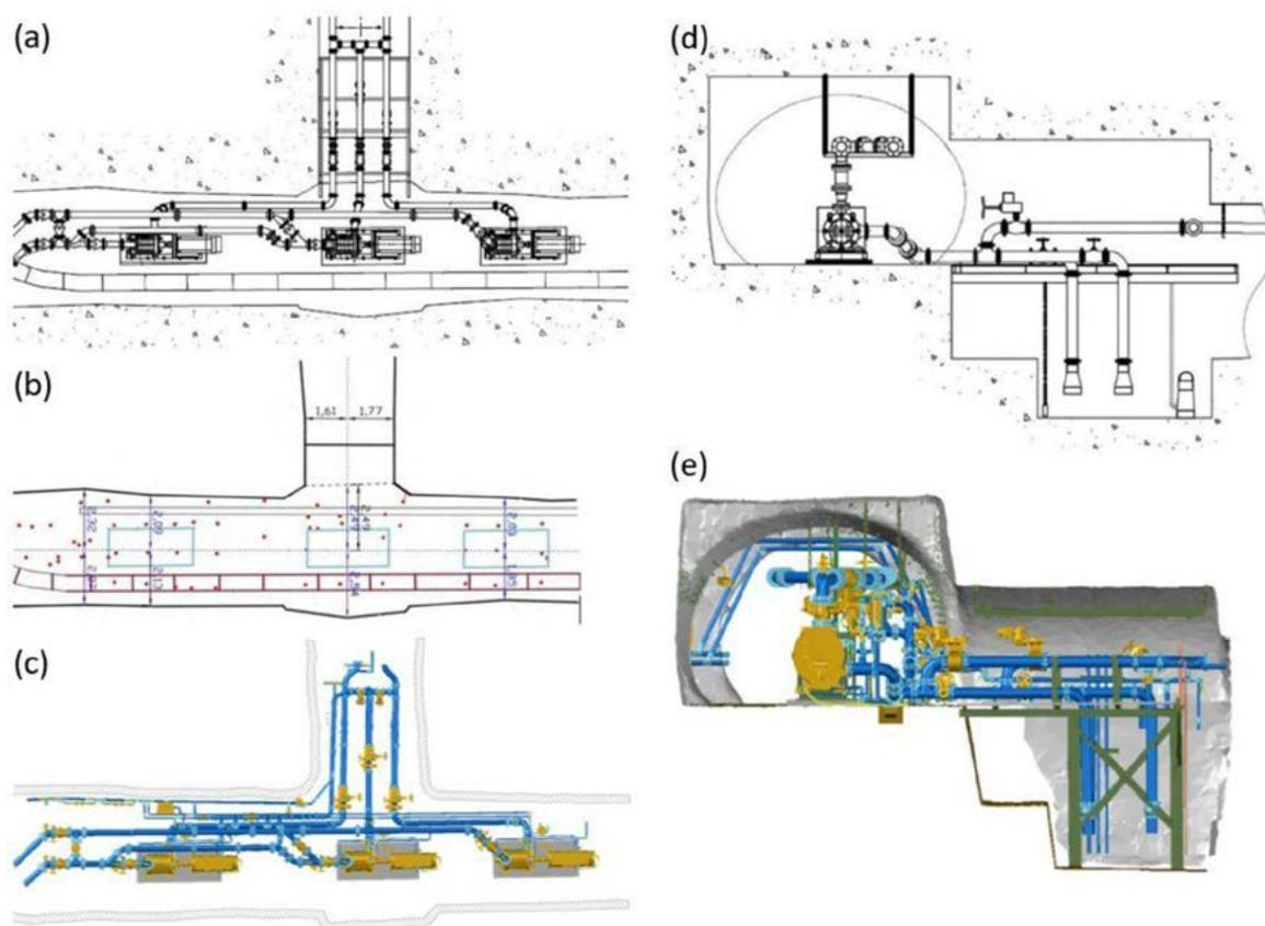
**Figure 8:** Comparison of engine room ground plan and cross section of design model and actual state after completion: (a) and (d) AutoCAD design model; (b) theodolite measurement result; and (c) and (e) TLS modelling.
