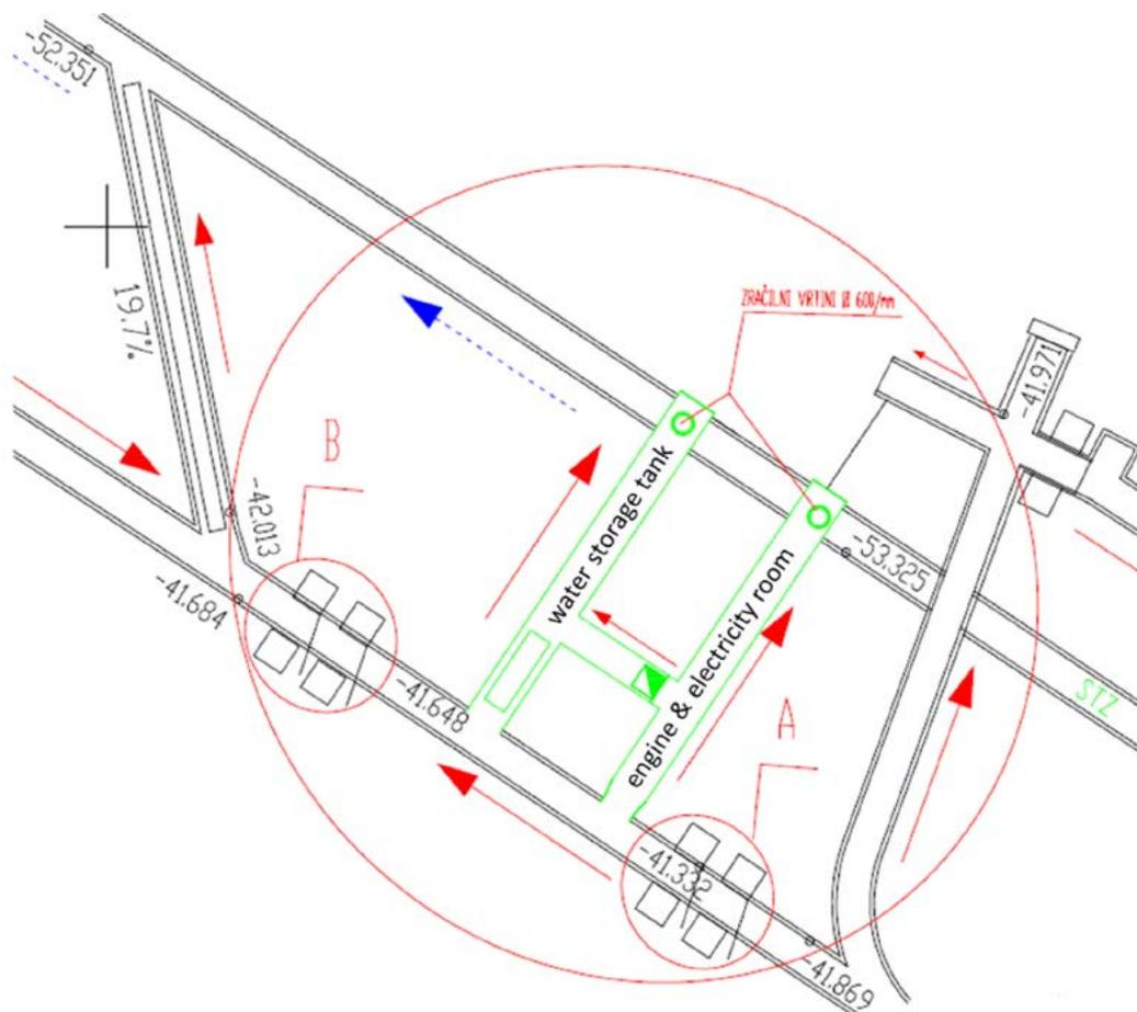
**Figure 1:** Location of underground pumping station (in green).
