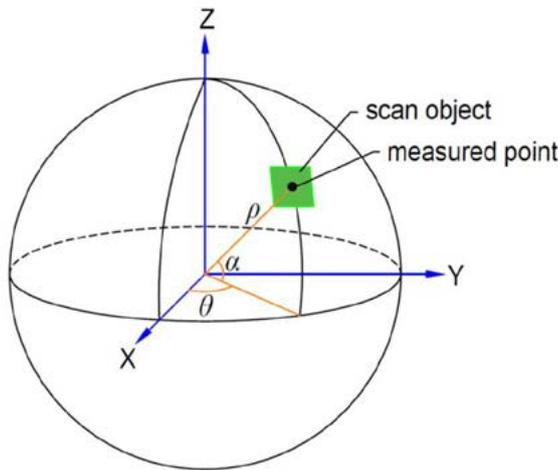
**Figure 2:** Spherical measuring system with a terrestrial laser scanner system.
