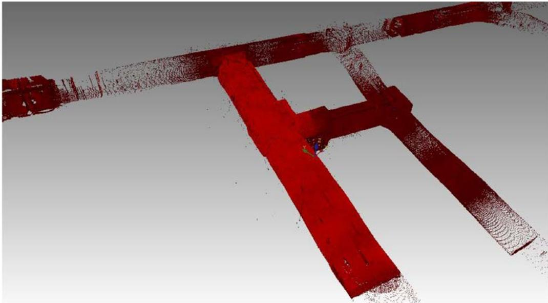
**Figure 5:** Resulting point cloud of 26 adjacent scans in the pumping station area.
