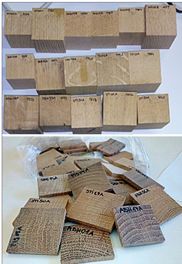
Slika 2. Kocke za določanje barve in gostote hrastovine (zgoraj) ter preizkušanci za določanje higroskopsnosti in dimenzijske stabilnosti (spodaj). Figure 2. Cubes for determining the colour and density of oak (top) and specimens for determining hygroscopicity and dimensional stability (bottom).
