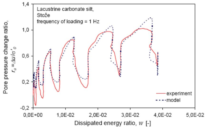
Figure 11. Pore-water pressure curve during an undrained cyclic triaxial test of lacustrine carbonate silt.
