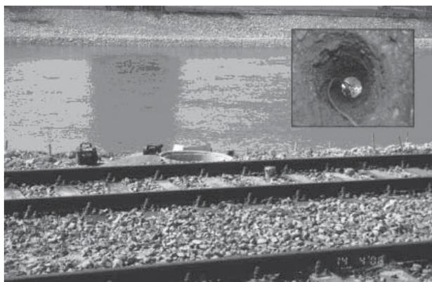
Figure 9. Railway embankment with a down-hole array and an accelerometer before the upheaval of the water.
