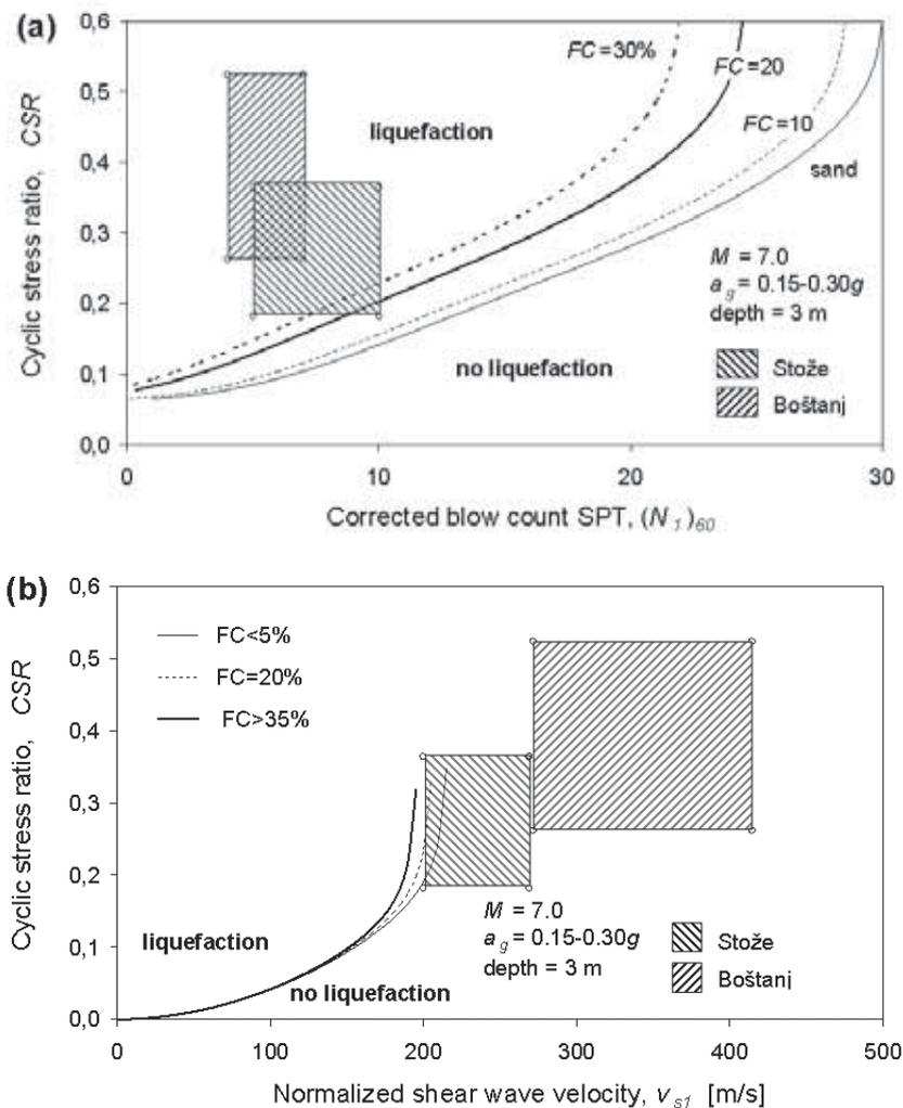
**Figure 2.** The danger of liquefaction occurring for silty sand from the Sava river and lacustrine carbonate silt from the Julian Alps. The CRR are based on (a) SPT measurements, (b) shear-wave velocity measurements.
