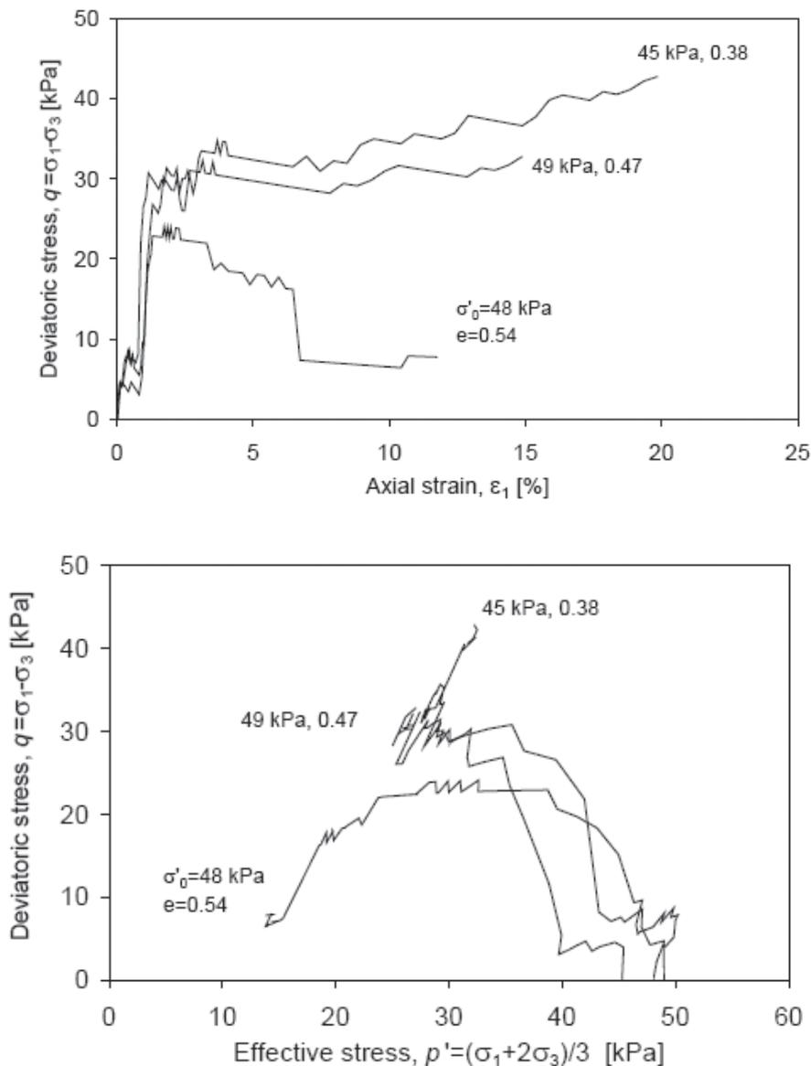
Figure 5. Undrained triaxial test of isotropic, consolidated, reconstituted samples of lacustrine carbonate silt from the Julian Alps.
