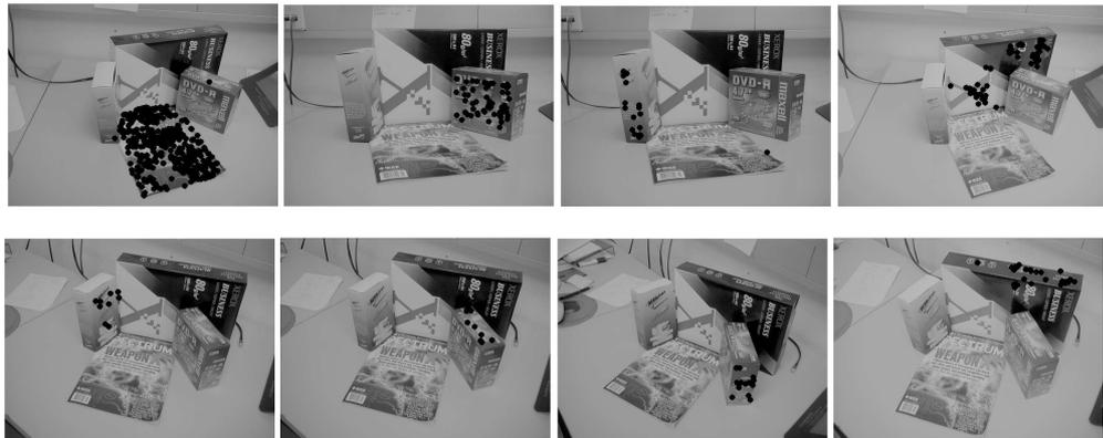
Figure 6. Experiment with a fixed scene. Eight clusters of SIFT features belonging to eight different planar parts of the scene are found.
