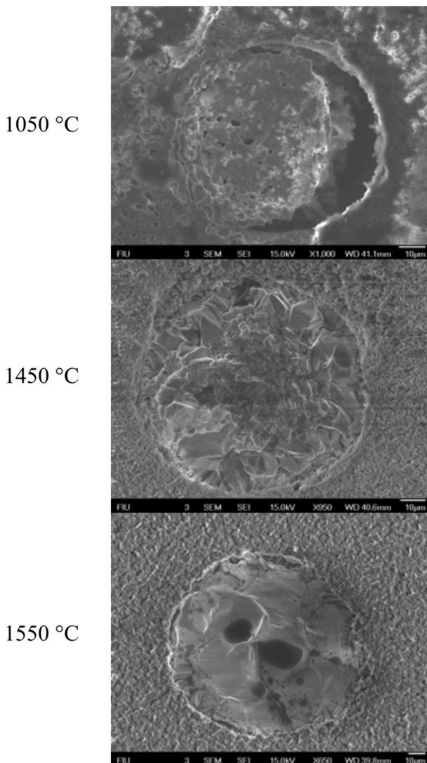
**Figure 11:** SEM image of the platinum particle via fired in different temperature
