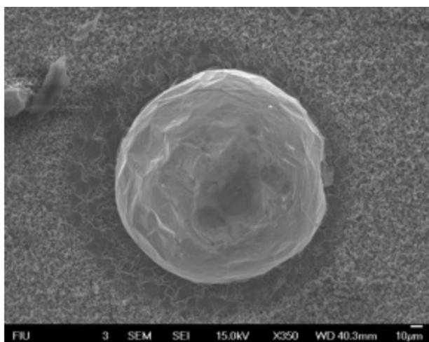
**Figure 12:** SEM image of the micron-sized platinum particle feedthrough via fired in 1550°C
