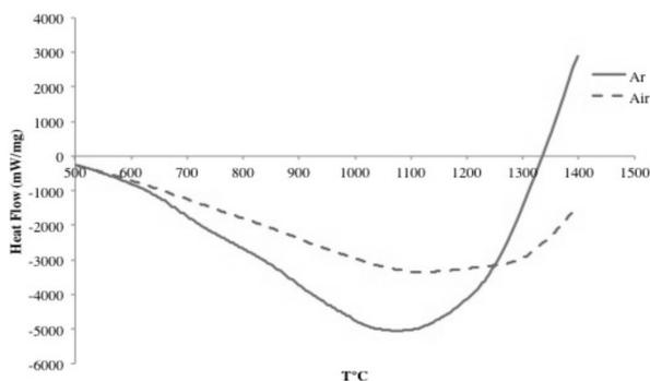
**Figure 6:** DSC analyses of the platinum powder in air and argon.
