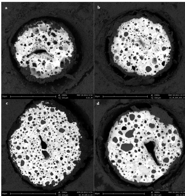
**Figure 2:** Backscatter SEM image of the platinum via fired in different heating rate. a) 0.2 °C/min, b) 1 °C/min, c) 5 °C/min and d) 20 °C/min.
