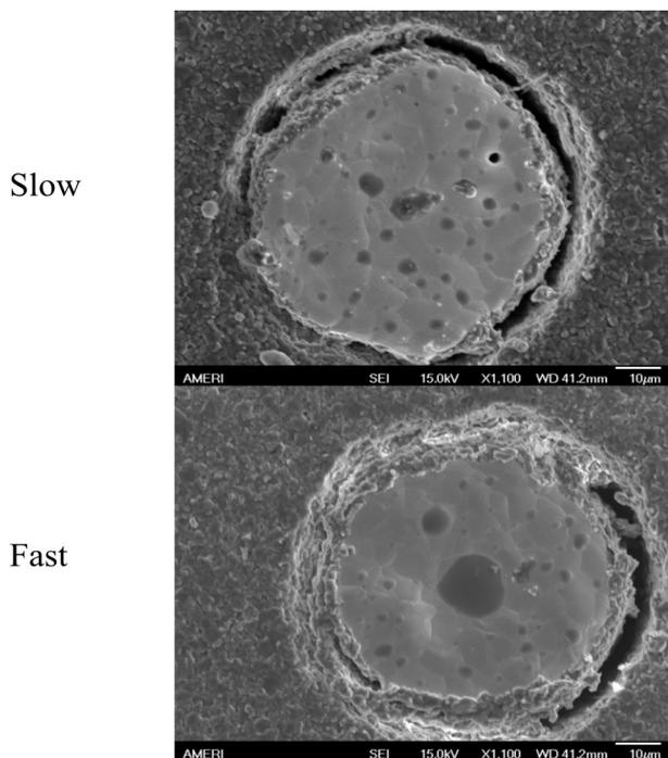
**Figure 9:** SEM image of the platinum particle via fired in different burn-out processes
