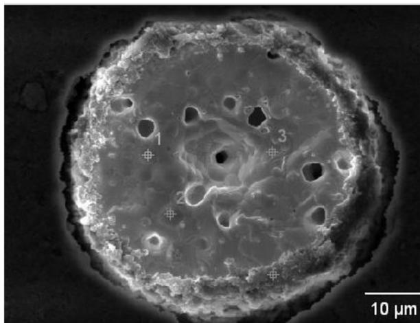
**Figure 3:** Backscatter image of Platinum Feedthrough fired in Air
