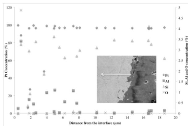
**Figure 13:** Concentrations gradient of different elements in platinum for the micron-sized platinum powder. Feedthrough fired in the H<sub>2</sub> – Ar (25-75) atmosphere at 1550 °C
