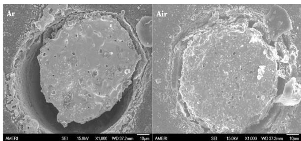
**Figure 5:** Secondary electron SEM image of feedthrough fired in air and argon atmosphere.
