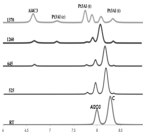
**Figure 8:** High temperature diffraction data of Pt/Alumina system
