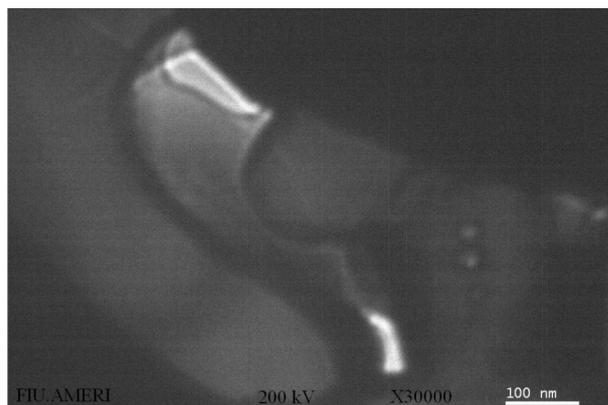
**Figure 10:** TEM image of the interface between platinum and alumina via fired ceramic particle.
