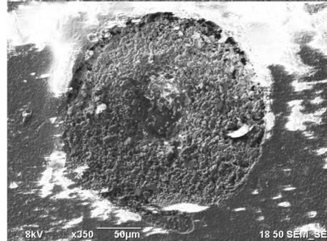
**Figure 4:** Microstructures of Platinum via with, 20%  $\text{Al}_2\text{O}_3$  in different via size
