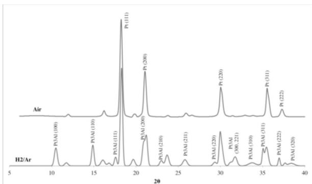
**Figure 7:** X-ray diffraction pattern of Platinum/ Alumina combination heated in two different environments in 1400°C
