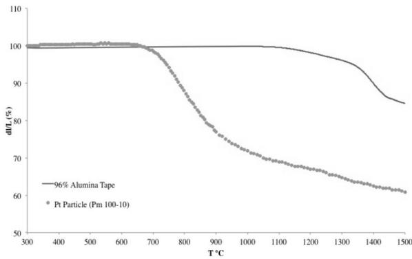
**Figure 1:** The nonisothermal densification behavior of platinum powder and alumina tape.
