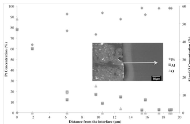
**Figure 14:** Concentration gradient of different element in platinum for the micron-sized platinum powder and 99.9% HTCC ceramic tape. Feedthrough fired in the H<sub>2</sub> – Ar (25-75) atmosphere at 1550 °C
