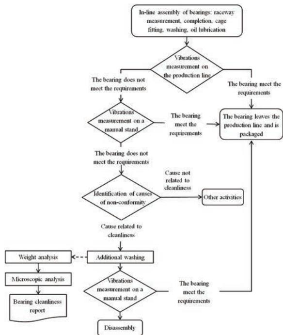
Fig. 1. Identification and evaluation of rolling bearing contamination in the quality control process
