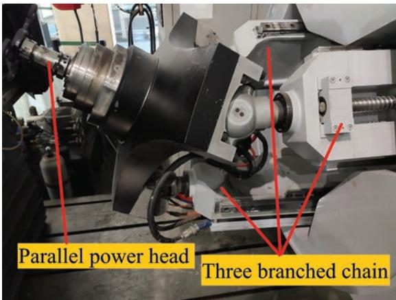
Fig. 7. 1T2R parallel power head
