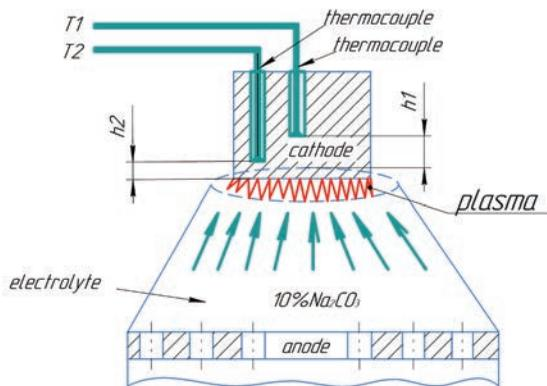
**Fig. 5.** The layout of thermal junctions in the surface layer of the sample when measuring the temperature in the process of electrolytic plasma heating
