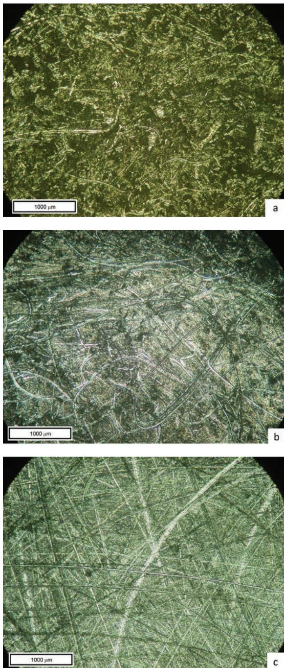
**Fig. 10.** Microrelief of 18CrNi3Mo-Sh steel samples after testing for abrasive wear resistance, 100 times increase; a) after EPP strengthening, b) thermo processed at VKMZ JSC, and c) initial state
