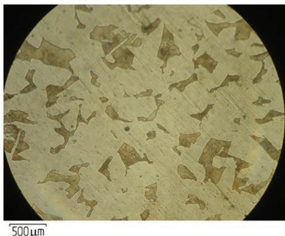
Fig. 3. The initial structure of the sample material of a component part of 18CrNi3Mo-Sh steel
