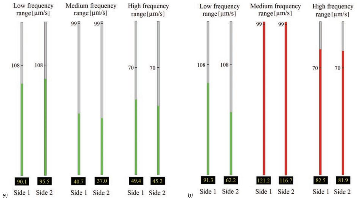
Fig. 3. a) Bar graph that shows the vibration level measurement of a bearing in good technical condition, and b) bar graph that shows the vibration level measurement of a bearing that does not meet the assumed quality control limits
