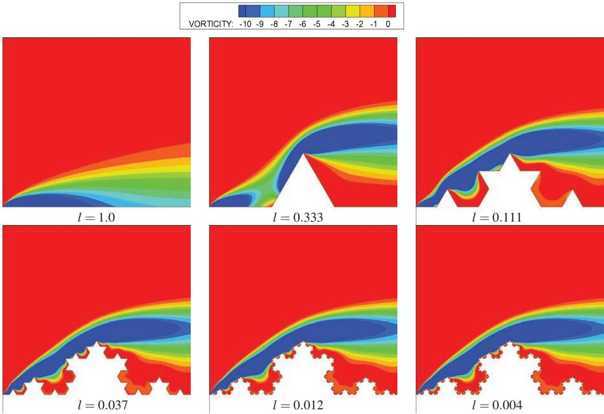
Fig. 9. Vorticity function contours for the Koch snowflake formation procedure denoted by fractal element length  $l$
