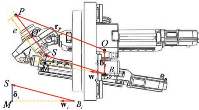
Fig. 3. Interference position of 1T2R spindle head
