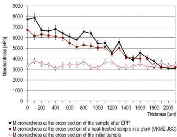
Fig. 9. The value of the microhardness of 18CrNi3Mo-Sh steel after EPP strengthening
