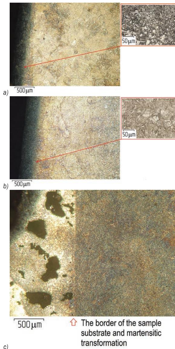
**Fig. 4.** Micro sections of the cross-section (to the depth of material) of electrolytic plasma processed steel
