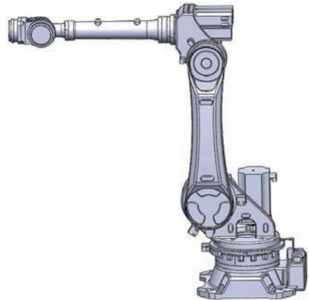
Fig. 2. The three-dimensional model of the manipulator
