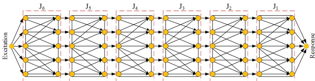
Fig. 1. Vibration Transfer model of the manipulator
