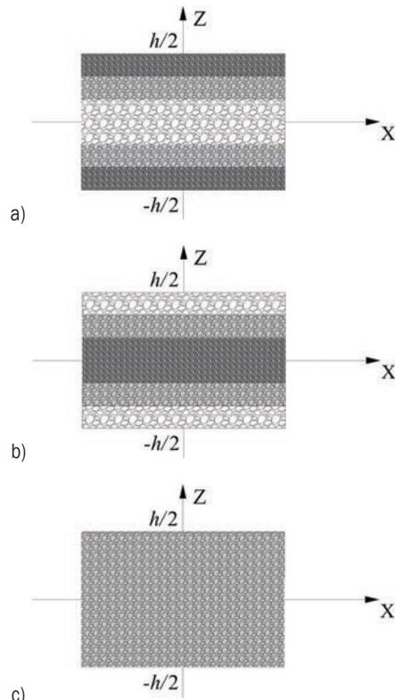
Fig. 2. Three types of porosity distributions; a) P-1, b) P-2, and c) P-3
