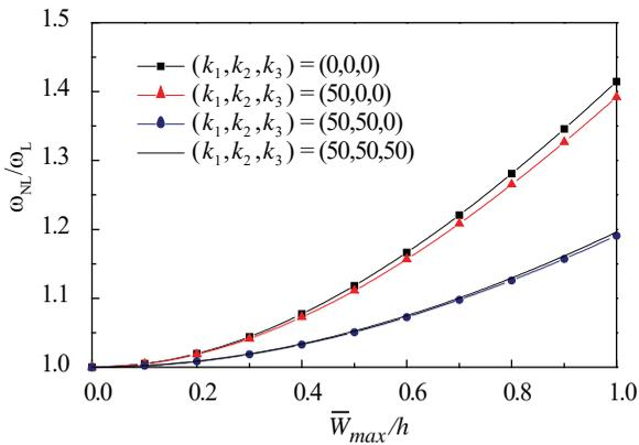
**Fig. 9.** Effect of elastic foundation on the frequency ratio for G-3/P-3
