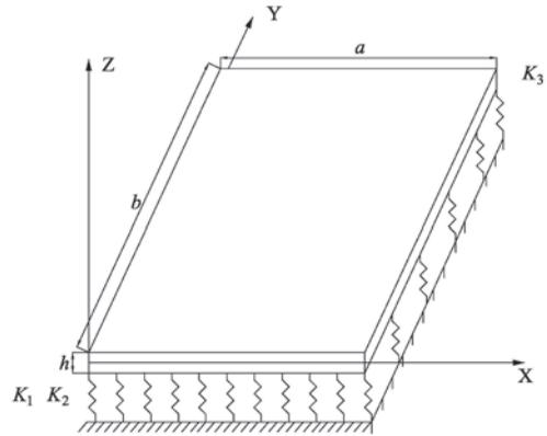
Fig. 1. A functionally graded GPL-reinforced porous plate on a nonlinear elastic foundation
