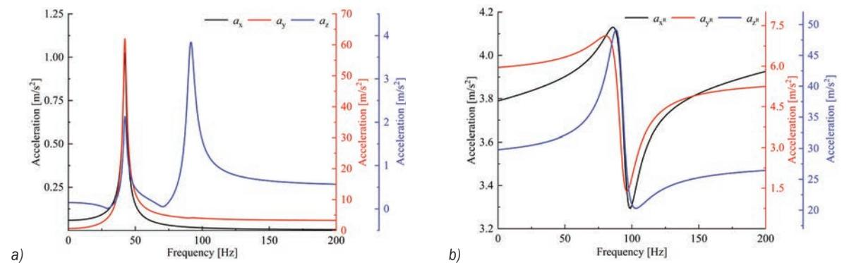
Fig. 7. Frequency responses curve of  $J_3$ ; a) translational acceleration, and b) rotational acceleration
