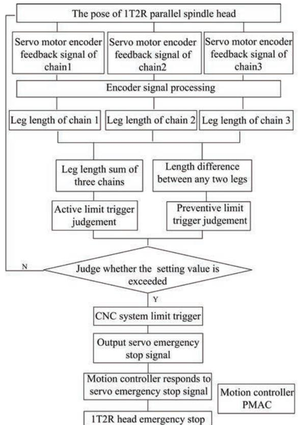
Fig. 6. Schematic diagram of limit protection process
