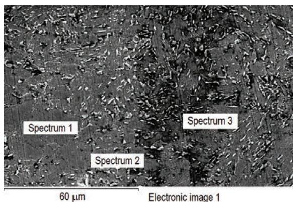
**Fig. 6.** Raster elemental analysis of the 18CrNi3Mo-Sh steel surface after EPP strengthening
