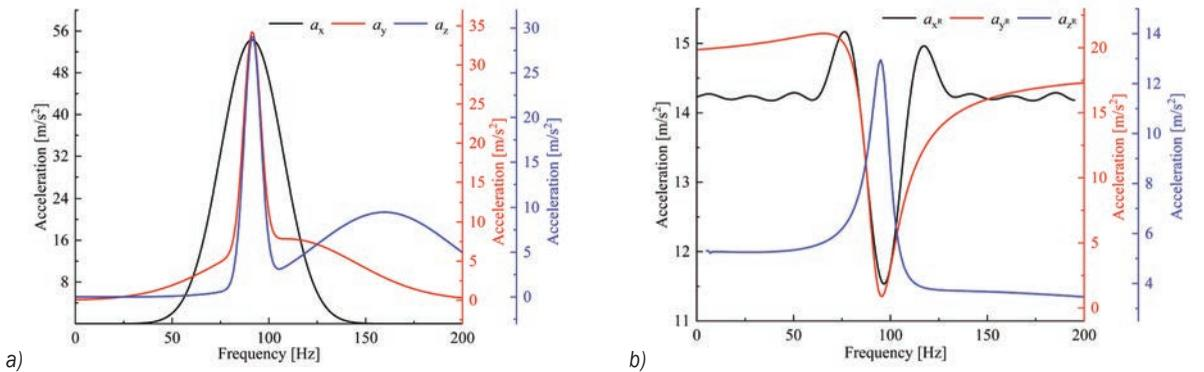
**Fig. 10.** Frequency response curves of  $J_6$ ; a) translational acceleration, and b) rotational acceleration
