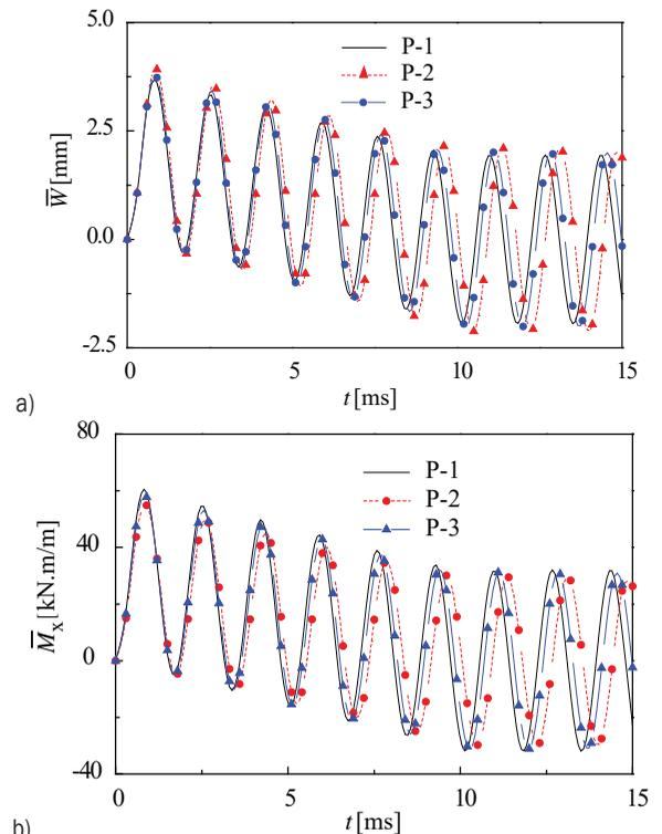
**Fig. 12.** Effect of porosity distributions on the transient responses for G-3; a) dynamic deflection, and b) dynamic bending moment
