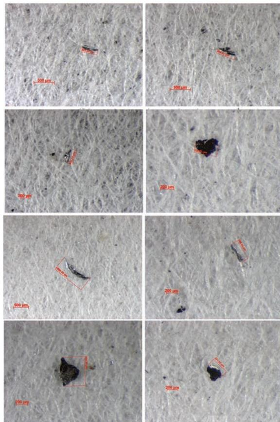
**Fig. 4.** Examples of microscopic photos of the filters showing contamination of the rolling bearings
