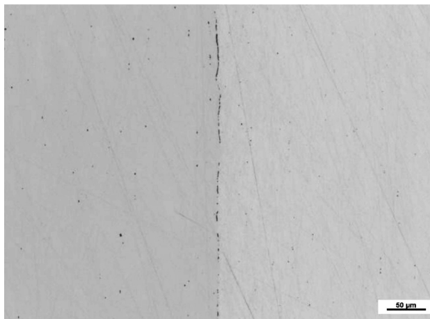
Figure 3: Joint between the 55C15N steel layer and AISI 304 steel layer; un-etched microstructure
