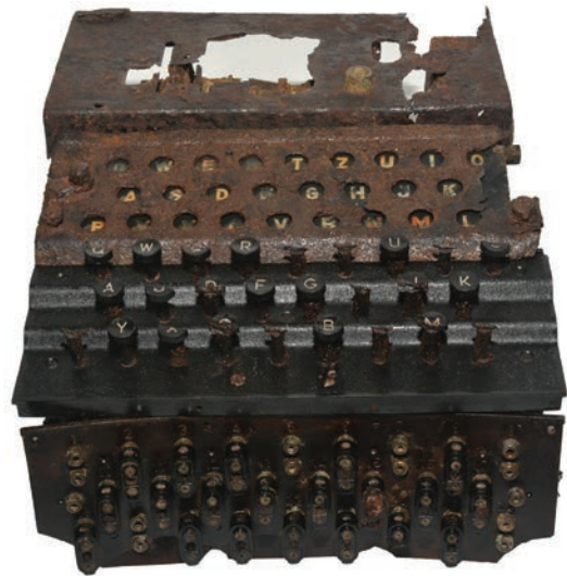
Figure 8: The remains of the Enigma M4 from the minesweeper R 15 after conservation (Photo: A. Gaspari).
