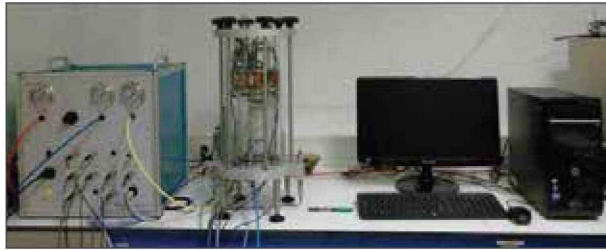
Figure 1. Resonant-column apparatus manufactured by Wykeham Farrance.
