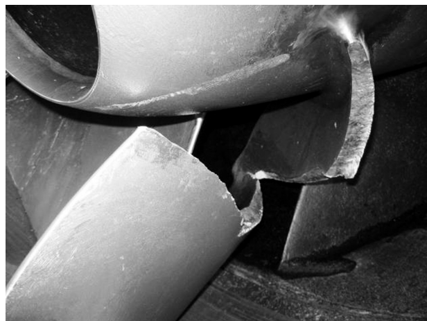
Figure 2: Damaged impeller blade
