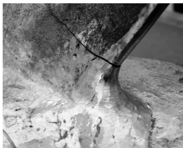
Figure 5: Crack at the leading edge of the blade
