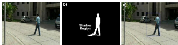
Figure 6: Moving object segmentation for an outdoor scene a) Original frame b) foreground mask c) bounding box representation of object.
