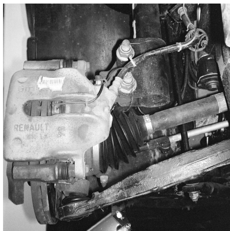
Sl. 11. Sprednja obesa vozila Renault safrane 2.2 RT Fig. 11. Front suspension of the Renault Safrane 2.2 RT
