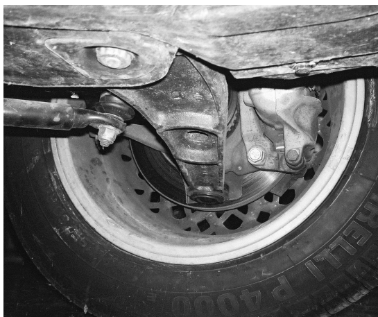
Sl. 11. Sprednja obesa vozila Renault safrane 2.2 RT Fig. 11. Front suspension of the Renault Safrane 2.2 RT
