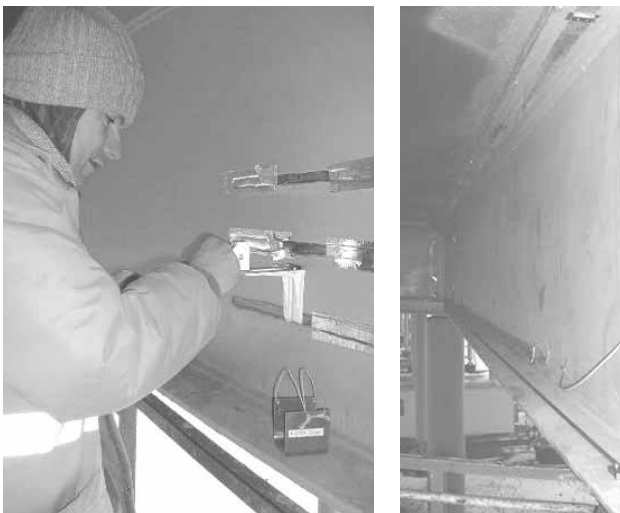
Fig. 16: On-site test of SMARTape gluing procedure (left) and installed SMARTapes.
