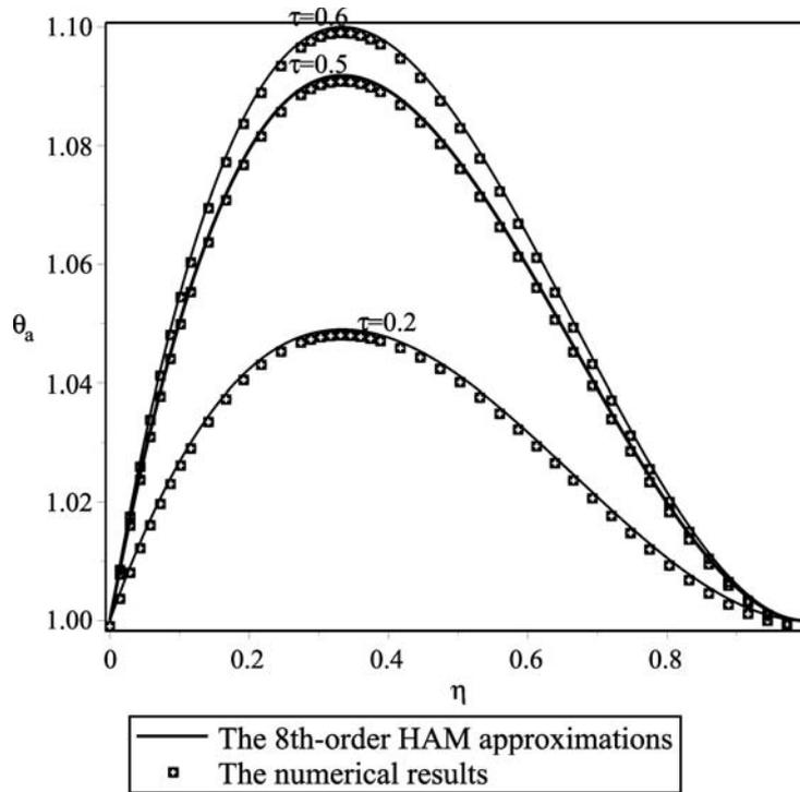
Figure 5. The 8<sup>th</sup>-order HAM approximations of  $\theta_a$  at  $\tau = 0.2, 0.5, 0.6, \alpha = 2, I = 10, h = -0.001$  open circle: the numerical results.
