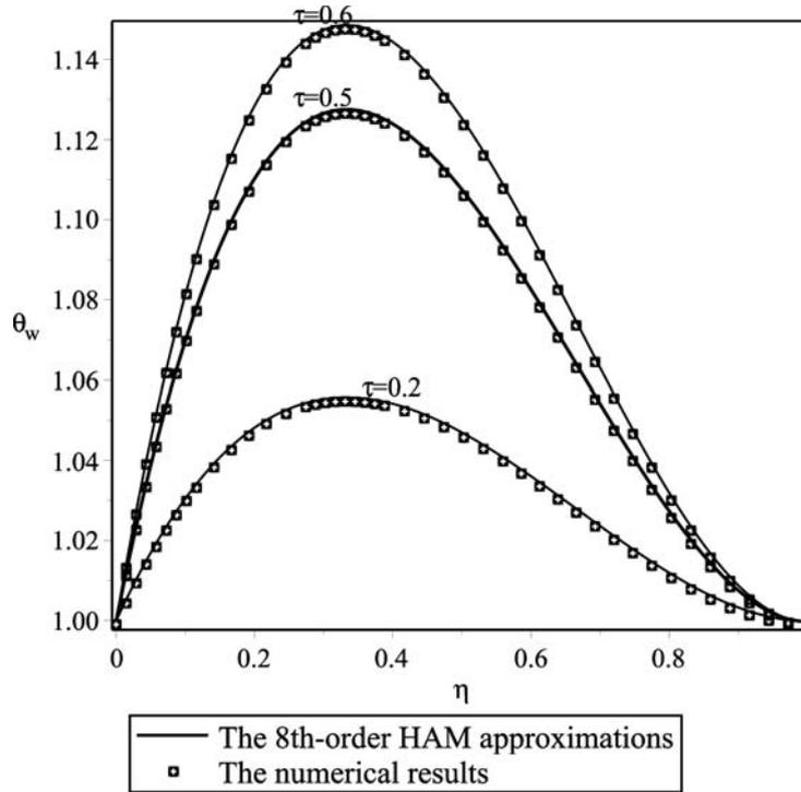
Figure 4. The 8<sup>th</sup>-order HAM approximations of  $\theta_w$  at  $\tau = 0.2, 0.5, 0.6, \alpha = 2, I = 10, h = -0.001$  open circle: the numerical results.
