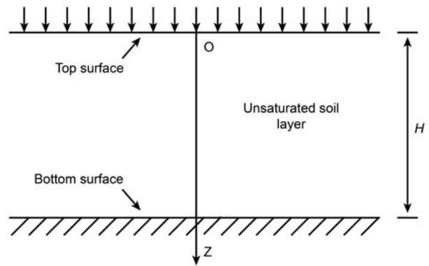
Figure 1. One-dimensional consolidation in unsaturated soils with a permeable top surface and an impermeable bottom base.
