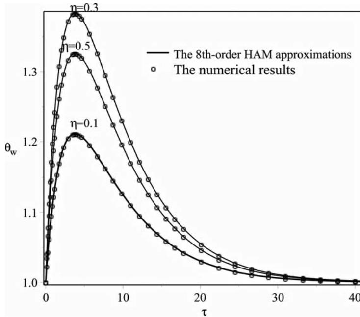
Figure 2. The 8<sup>th</sup>-order HAM approximations of  $\theta_w$  at  $\eta = 0.1, 0.3, 0.5$ ,  $\alpha = 2$ ,  $I = 10$ ,  $h = -0.001$  open circle: the numerical results.
