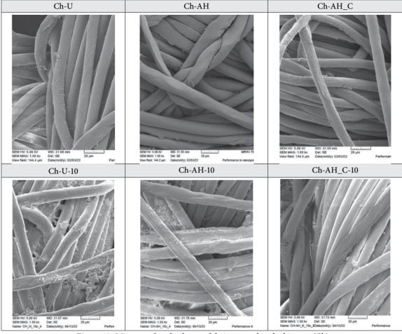
*Figure 10: Micrographs of polyester fabrics coated with chitosan (Ch) before and after washing (Ch-U-10, Ch-AH-10, Ch-AH\_C-10) magnified 1,500-×*
