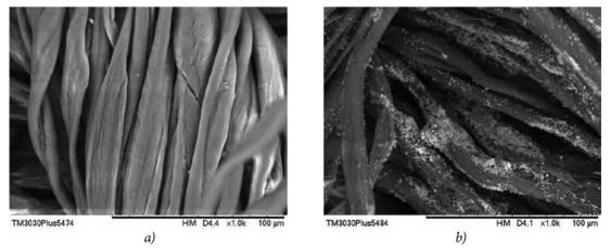
Figure 5: SEM images of cotton fibre (1000× magnification): (a) untreated with TiO<sub>2</sub>; (b) treated with TiO<sub>2</sub>
