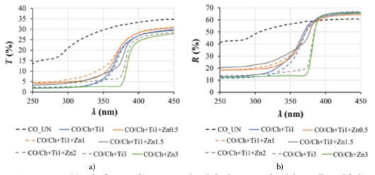
Figure 5: Transmittance (a) and reflectance (b) versus wavelength for the untreated and chemically modified samples
