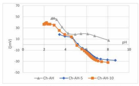
Figure 5: Zeta potential of chitosan-alkali hydrolysed PES fabrics before and after washing cycles in variations of pH 1 mmol/L KCl
