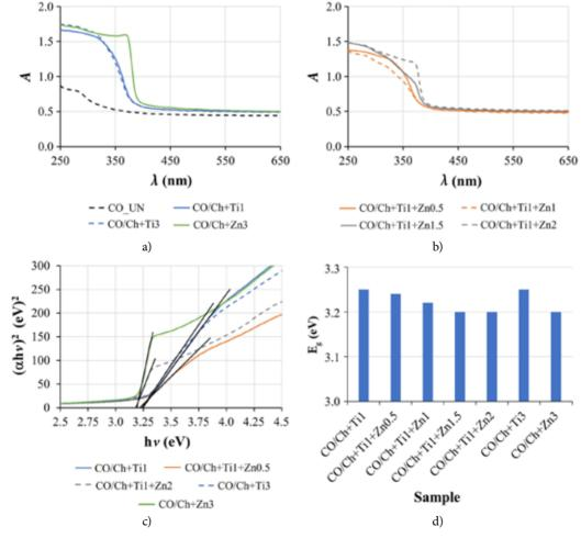
Figure 4: Absorption spectra of the untreated and functionalised cotton samples (a, b); Tauc plots of the representative samples (c) and  $E_g$  values of the functionalised cotton sample
