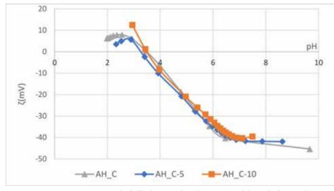
Figure 6: Zeta potential of alkali treated with promoter fabrics before and after washing cycles in variations of pH 1 mmol/L KCl
