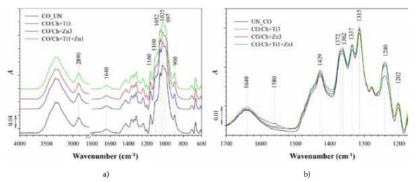
Figure 3: IR ATR spectra of the untreated cotton sample (CO\_UN) and the chemically modified CO/Ch+Ti1+Zn1, CO/Ch+Ti3, and CO/Ch+Zn3 samples in the spectral region of 4000–600 cm<sup>-1</sup> (a) and in the spectral region of 1700–1180 cm<sup>-1</sup> (b)
