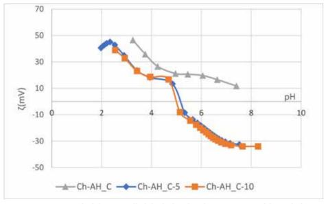
Figure 7: Zeta potential of chitosan-alkali hydrolysed with promoter PES fabrics, before and after washing cycles in variations of pH 1 mmol/L KCl
