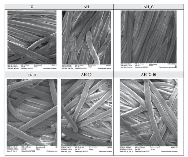
*Figure 9: Micrographs of control (U) and modified polyester fabrics (AH, AH\_C) before and after washing (U-10, AH-10, AH\_C-10) magnified 1,500-×*
