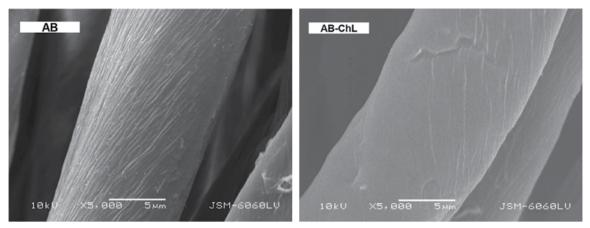
*Figure 2: SEM images of surface of alkaline-scoured and bleached cotton yarns (AB) treated with 0.6% concentration of chitosan solution (AB-ChL)*
