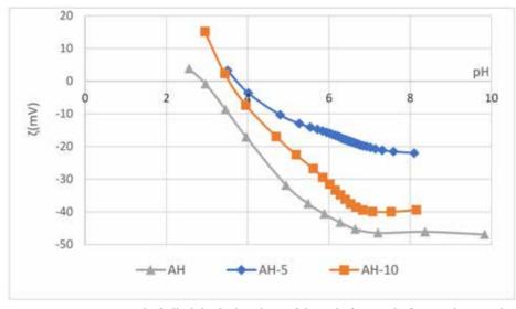
*Figure 4: Zeta potential of alkali hydrolysed PES fabrics before and after washing cycles in variations of pH 1 mmol/L KCl*
