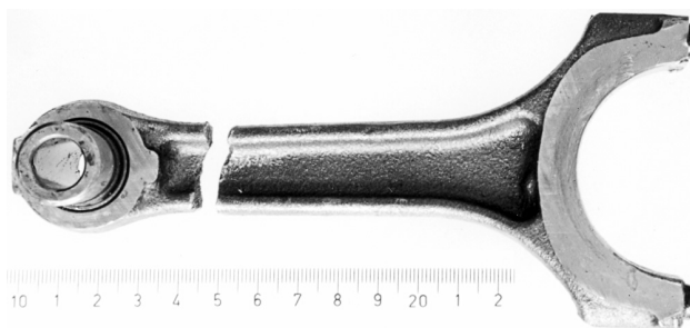
Figure 1: Connecting rod's fractured shank
