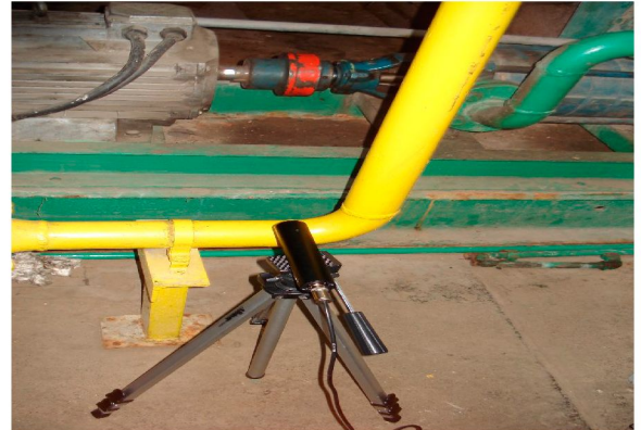
Figure 4: Tachometer positioning manner for recording output shaft speed.
