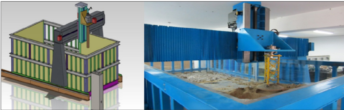
Figure 2. Pile-soil interaction experimental facility.
