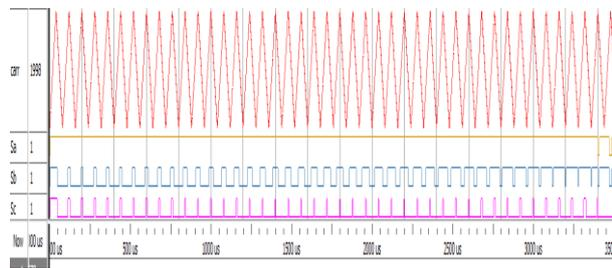
Figure 11. Generated switching for Sector I (V100-V110).
