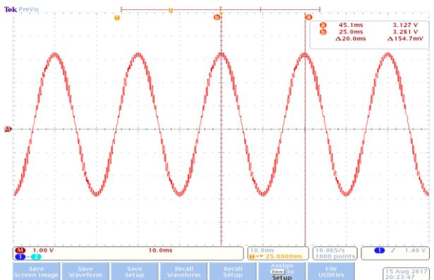
Figure 15. Experimental results of three filtered line-to-neutral output voltages (Sa-Sb).
