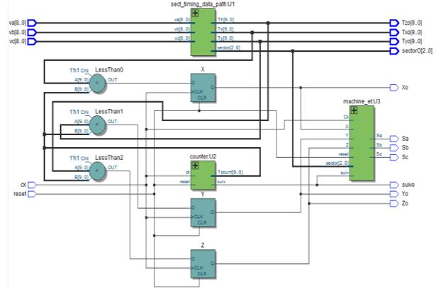
Figure 8. RTL view of the optimized SVPWM.
