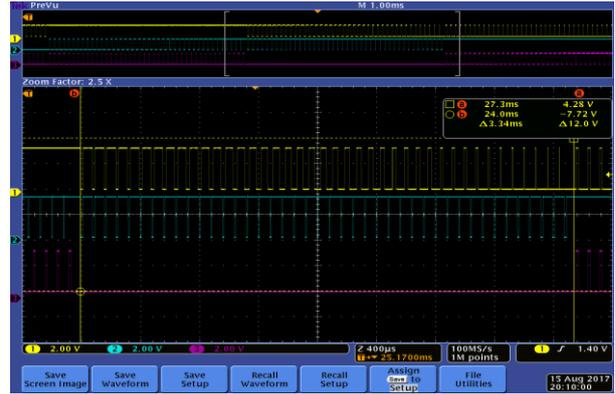
Figure 13. Generated switching pulses for Sector 6.
