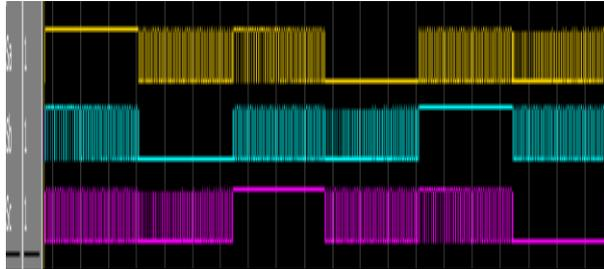
Figure 10. Global simulation results of the SVPWM generator.
