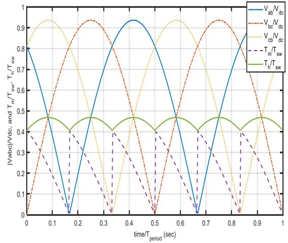
Figure 4. Switching times for Balanced three-phase pattern with a 50% modulation depth.
