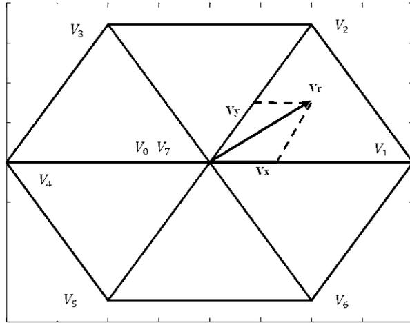
Figure 2. Principle drawing SVM for a three-phase two level-VSI.
