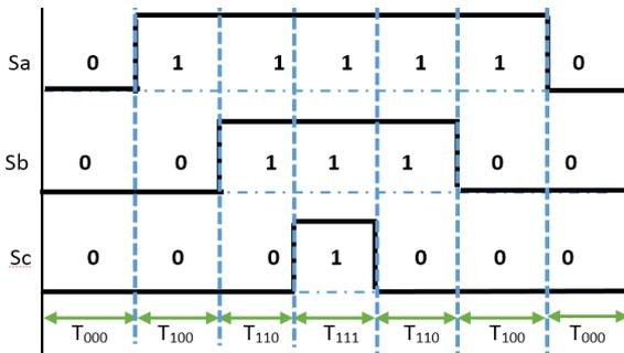
Figure 3. Switching-time pattern for Sector I.
