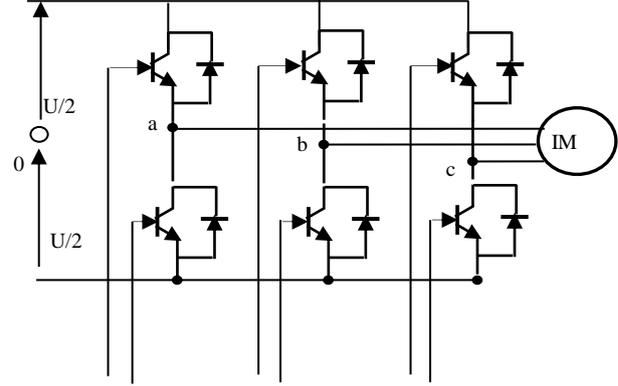
Figure 1. Two level controlled voltage source inverter.
