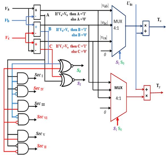
Figure 5. Sector selector and timing of the active vectors.
