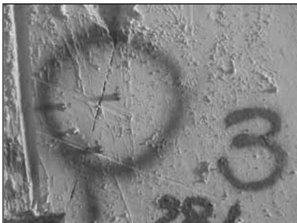
Figure 21. Manual measurement of the displacements of open dikes within safety pillars.
