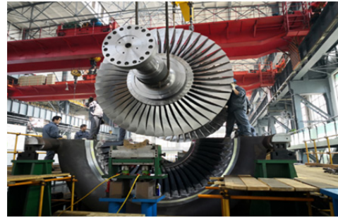
Fig. 2 Typical working situation of ETO assembly
