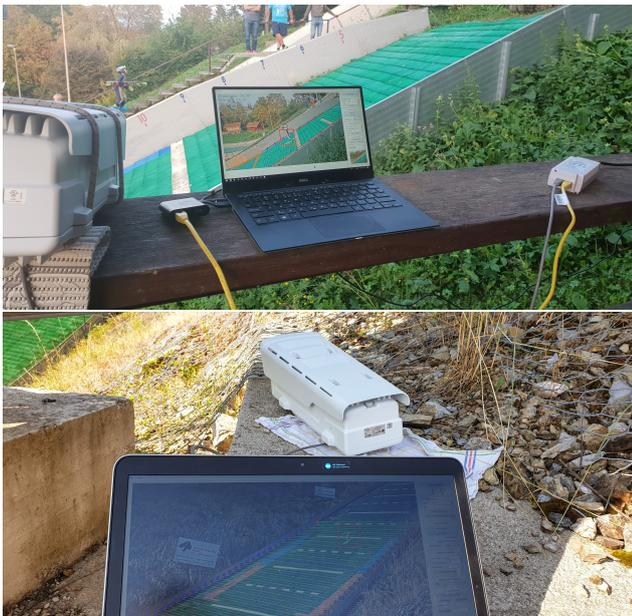
Figure 7: Measurement system in action at the HS=109 m hill in Kranj (bottom) and HS=21 m hill in Mengeš (top), Slovenia. The laptop and the camera are connected using a PoE switch.
