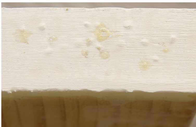
Fig. 3: Blisters formed at a temperature of 82.7 °C on the front side of the sample, and leakage of the resin
