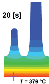
Figure 9: Optimized intermediate cooling rib during an emergency stop scenario at t = 20 s
