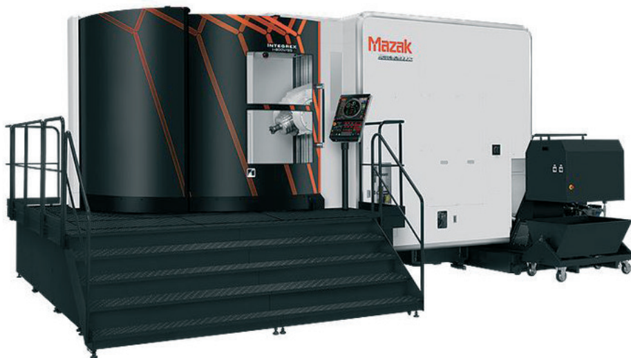
» The INTEGREX i-800V/8 combines full 5-axis milling, powerful turning operations and pallet-changing capabilities to quickly process large, highly complex parts.
