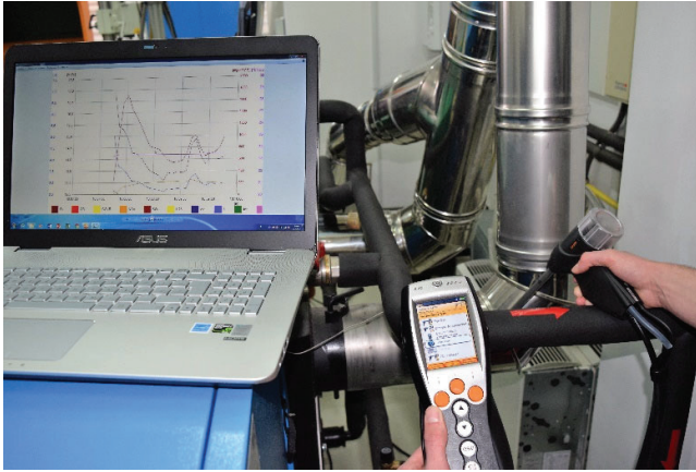
Figure 8: Fine particle measurement with the Testo 380 fine particle analyser
