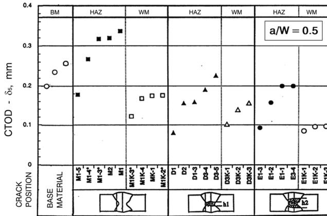
\*) Non uniform fatigue crack front profile
