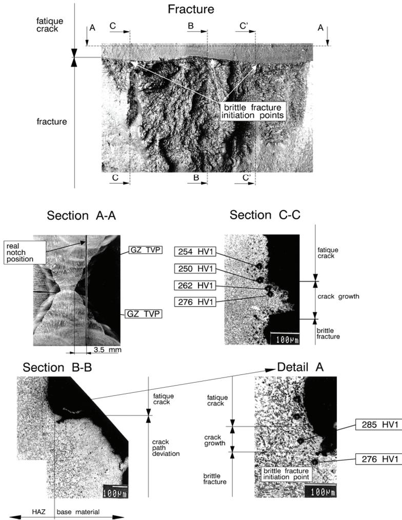
**Figure 6:** Brittle fracture initiation points and crack path deviation on fractured specimen  $B \times 2B$  with deep cracks in HAZ of heterogeneous undermatched weld joint
