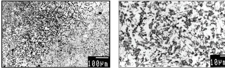
**Figure 4:** HAZ, heated at intercritical temperature between  $A_{c1}$  in  $A_{c3}$  (IC HAZ). At higher magnification, the region of partial transformation to austenite, from which M-A constituents are formed, can be seen.
