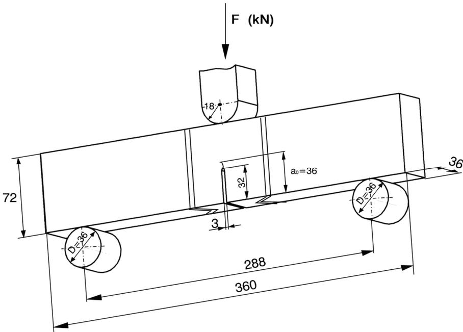
**Figure 1:** Shape and dimensions, and loading conditions for bend SENB specimens ( $B \times 2B$ ), made from homogeneous and heterogeneous undermatched weld joints
