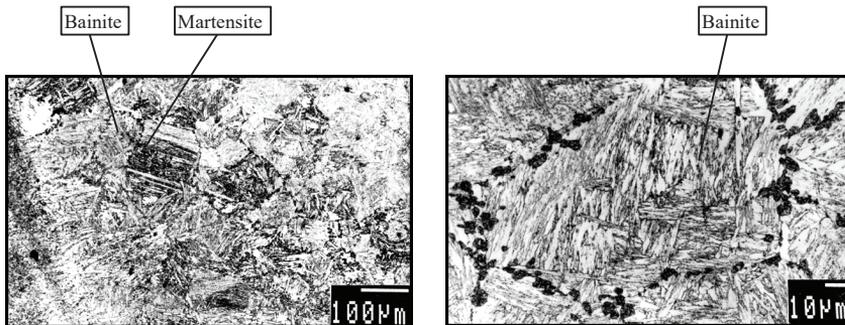
**Figure 3:** CG HAZ with bainitic-martensitic microstructure, which was subsequently heated at a temperature between  $A_{c1}$  and  $A_{c3}$ , i.e., IC CG HAZ b) with distributed brittle M-A constituents along grain boundaries of primary grains (ASTM 4) with directed bainitic microstructure.
