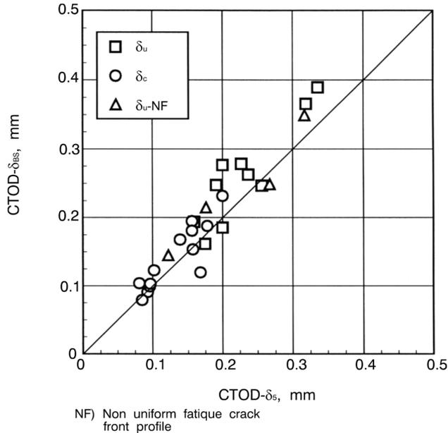
**Figure 7:** Comparison of directly measured ( $\delta_5$ ) and calculated ( $\delta_{BS}$ ) CTOD fracture toughness values of specimens  $B \times 2B$  with deep crack ( $a/W = 0.5$ ) in homogeneous and heterogeneous undermatched weld joints
