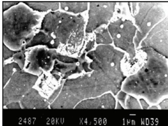
**Figure 8:** Mainly ferritic microstructure with carbides (Fe<sub>3</sub>C) precipitated at the HAZ grain boundary
