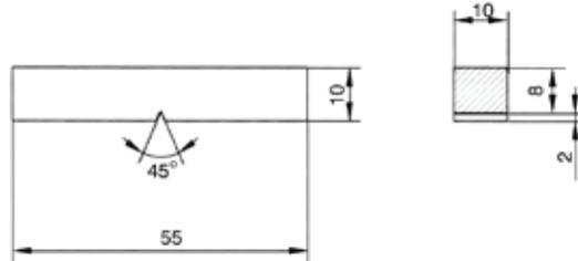
**Figure 5:** Shape and dimensions of Charpy – V notch specimen
