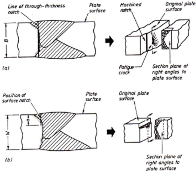
**Figure 3:** Example of sectioning techniques for
