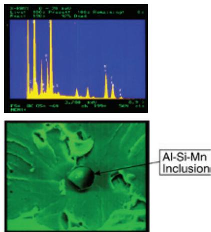
**Figure 9:** Appearance and EDX analysis of brittle fracture initiation point, i.e. Al-Si-Mn inclusion in the HAZ specimen
