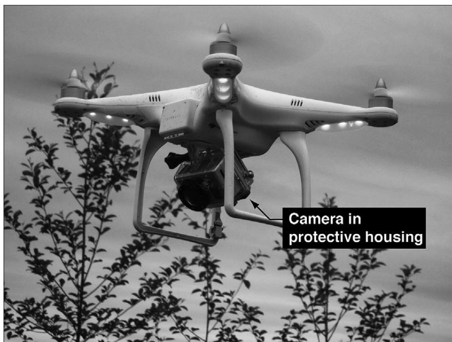
Fig. 1: Mini multi-rotor UAVs equipped with compact high-resolution cameras are inexpensive and have the potential to increase data collection and monitoring capacity for karst researchers and managers (Photo: C.L. Ramsey).
