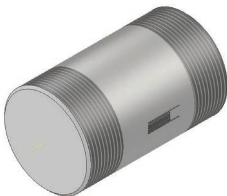
Fig. 5. Locations of the strain gauges on the central pin
