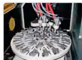
Automatic and controlled blasting process
