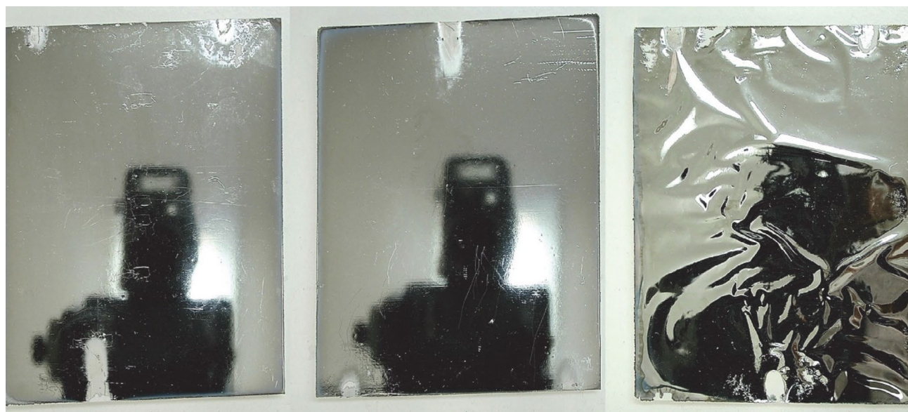
Figure 6. White-ABS premetalized with Ni-JetMetal® and electrolytic deposition of Cu-Ni-Cr: (a) sulfuric-chromic bath for 10 min; (B) sulfuric-chromic bath for 15 min; (C) \text{KMnO}_4 for 15 min.
