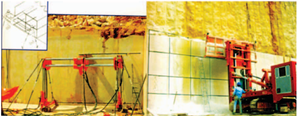
Figure 7. Comparison of initial cuts for a gallery with both Fantini machines [4]
