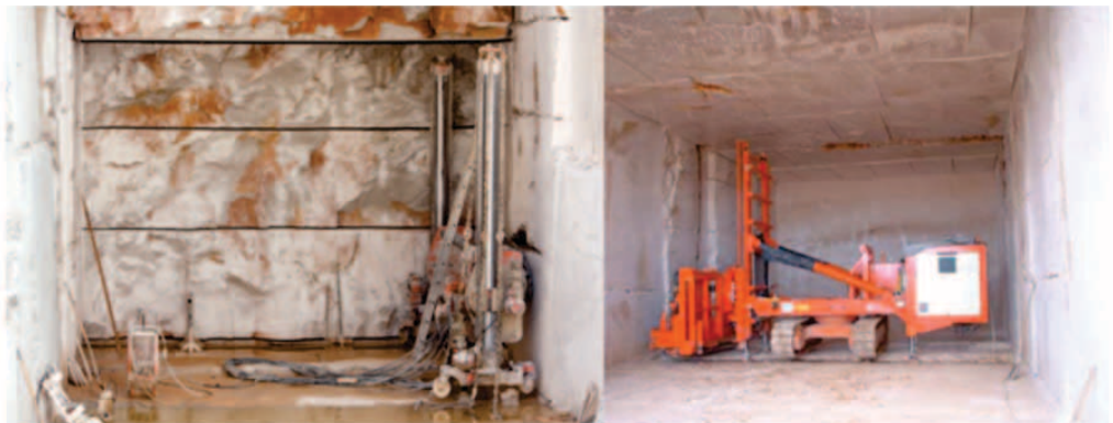
Figure 3. An old and a new model of the chain saw machine for underground mining. Left: the Fantini G. 70 model on fixing pillars. Right: the new Fantini GU 70/R model. [6]
