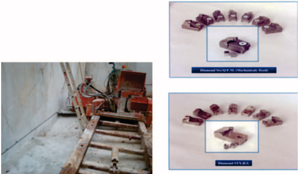
Figure 2. A track chain saw and cutting elements [6]
