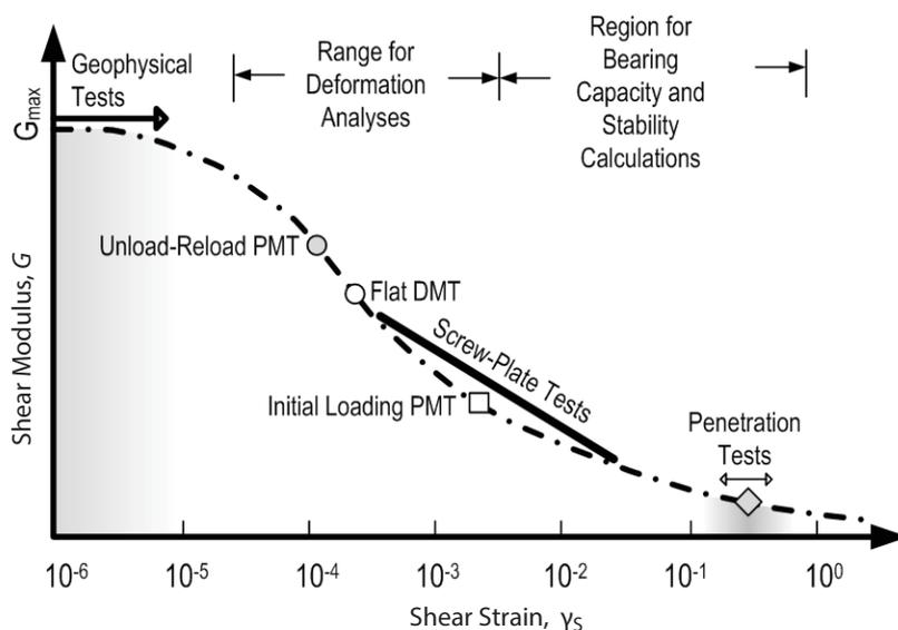
**Figure 1.** The starting point of the stress-strain curve (at low strain  $\gamma_S \sim 10^{-6}$ ) can be accurately established from seismic tests and its end point (at high strain  $\gamma_S \sim 10^{-1}$ ) by dynamic tests [12].
