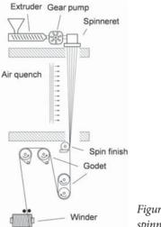
*Figure 1: Lab scale melt spinning plant*
