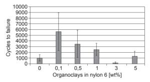
Figure 3: Abrasion resistance with bechlenberg
