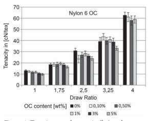
*Figure 4: Tenacity over draw ratio*  $(\lambda_D)$  *and organoclay (OC) content*
