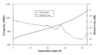
Fig. 6. The effect of different separation angel,  $\Theta$  on resonant frequency and return loss
