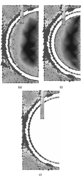
Fig. 4. Current distribution at 920MHz of (a) half annular ring slot antenna (b) half double annular ring slot antenna and (c) half double annular ring slot antenna without central disk
