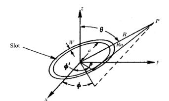
Fig. 1. Annular-slot Geometry
