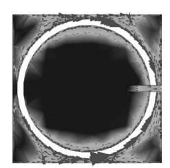
Fig. 3. Current distribution at 920MHz of (a) conventional annular ring slot antenna and (b) annular ring slot antenna with side feeding
