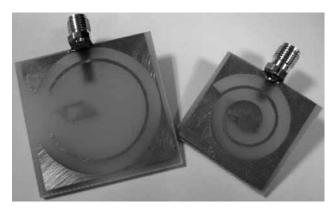
Fig. 9. Fabricated Prototype of the designed antennas shown in Figure 5
