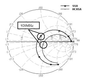
Fig. 12. The input impedance of the miniaturized proposed antennas
