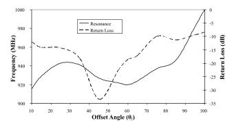
Fig. 7. The relationship between the offset angle,  $\Theta_{\rm f}$  with resonance and return loss
