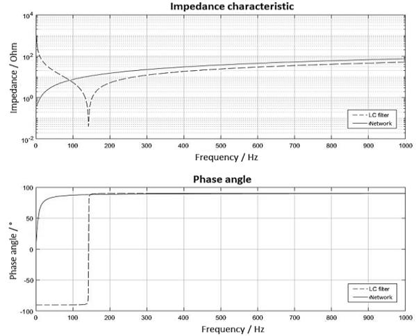
Figure 7. Frequency impedance characteristic of the load (three parallel  $RLC$  circuits on the load side) and the system side using the ITM interface algorithm (Matlab Simulink).
