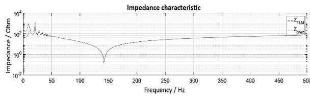
Figure 9. Impedance characteristic of the load side ( $RLC$  load) of the system using the TLM interface algorithm compared to the impedance characteristic of the load (Matlab Simulink).
