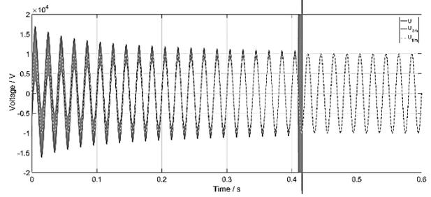
Figure 15. Simulation comparison of the voltages at a load connected to the system ( $t=0.2$  s) and at a transmission line outage at the system power decreased from 100 MVA to 75 MVA.
