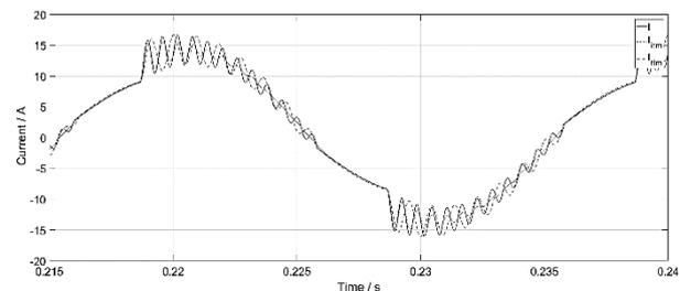
Figure 17. Simulation comparison of the currents at the load connected to the grid.
