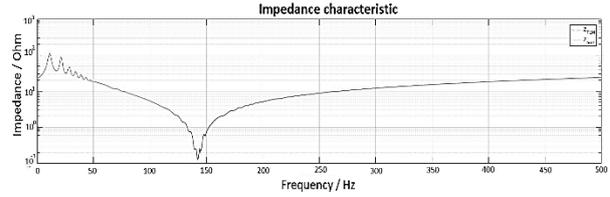
Figure 11. Impedance characteristic of the load side (three parallel  $RLC$  circuits on the load side) of the system using the TLM interface algorithm compared to the impedance characteristic of the load (Matlab Simulink).
