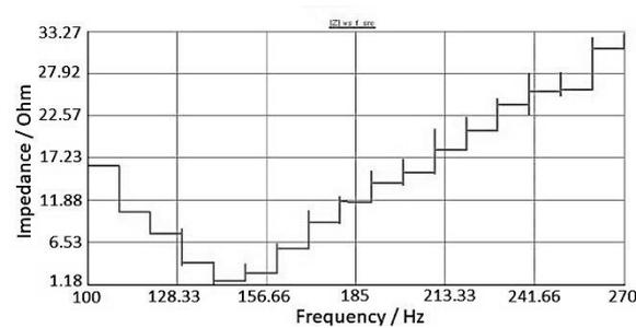
Figure 10. Impedance characteristic of the load side ( $RLC$  load) of the system (impedance of load, modelled on Typhoon HIL and observed from RTDS) using the TLM interface algorithm (RTDS).
