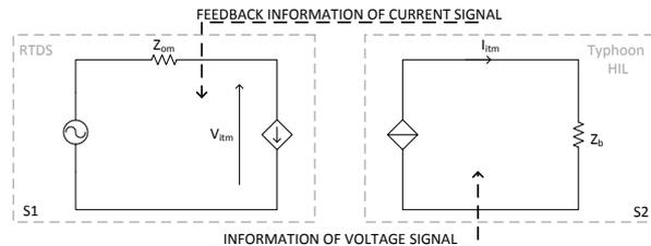
Figure 1. Ideal Transformer Model Interface scheme for the HIL simulation.
