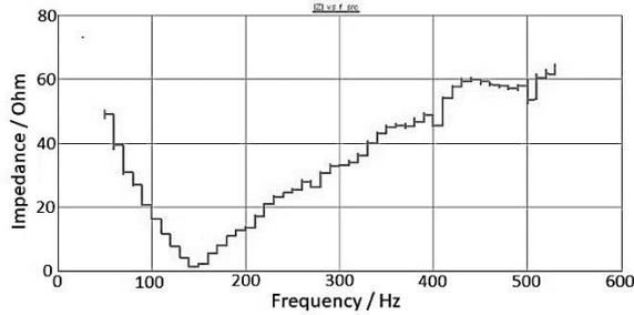
Figure 5. Impedance characteristic of the load side ( $RLC$  load) of the system (impedance of the load modelled on Typhoon HIL and observed from RTDS) using the ITM interface algorithm (RTDS).
