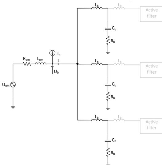
Figure 6. Topology of the second example for the HIL simulation using three parallel  $RLC$  load circuits.
