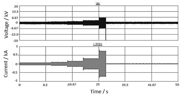
Figure 8. Voltage and current of the system using the ITM interface algorithm with three parallel  $RLC$  circuits on the load side during the systems transition to an unstable state.
