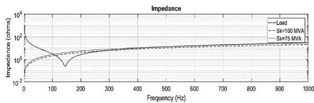
Figure 14. Impedance characteristic of the load side and impedance characteristic of the system.
