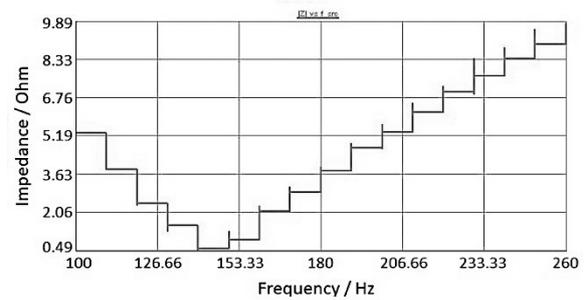
Figure 12. Impedance characteristic of the load side (three parallel  $RLC$  circuits on the load side) of the system (load impedance modelled on Typhoon HIL and observed from RTDS) using the TLM interface algorithm (RTDS).
