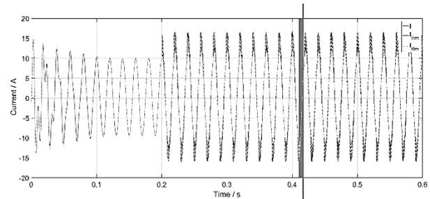
Figure 16. Simulation comparison of the currents at a load connected to the system ( $t=0.2$  s) and at a transmission line outage at the system power decreased from 100 MVA to 75 MVA.
