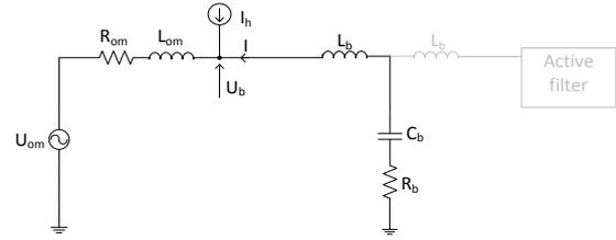
Figure 3. Topology of the first example for the HIL simulations using an RLC load circuit.
