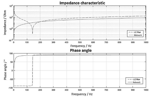
Figure 4. Frequency impedance characteristic of the load (RLC load) and the system side using the ITM interface algorithm (Matlab Simulink).
