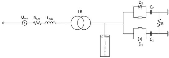
Figure 13. Topology of the network with a two-wire diode rectifier on the load side ( $U_{om} = 1$  p.u. (50 Hz),  $S_k = 100/75$  MVA,  $S_{tr} = 1$  MVA,  $S_{LC} = 0,1$  MVA,  $f_{LC} = 145$  Hz,  $C_1 = 100$   $\mu$ F,  $C_2 = 100$   $\mu$ F,  $R = 50$   $\Omega$ ).
