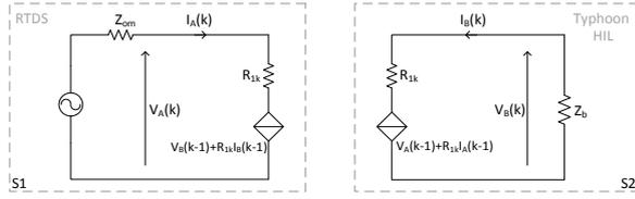
Figure 2. Transmission Line Model Interface scheme for the HIL simulation.
