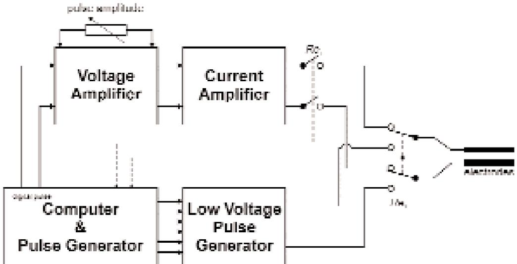
Figure 1. Block diagram of *in vitro* electroporator GT-1.
