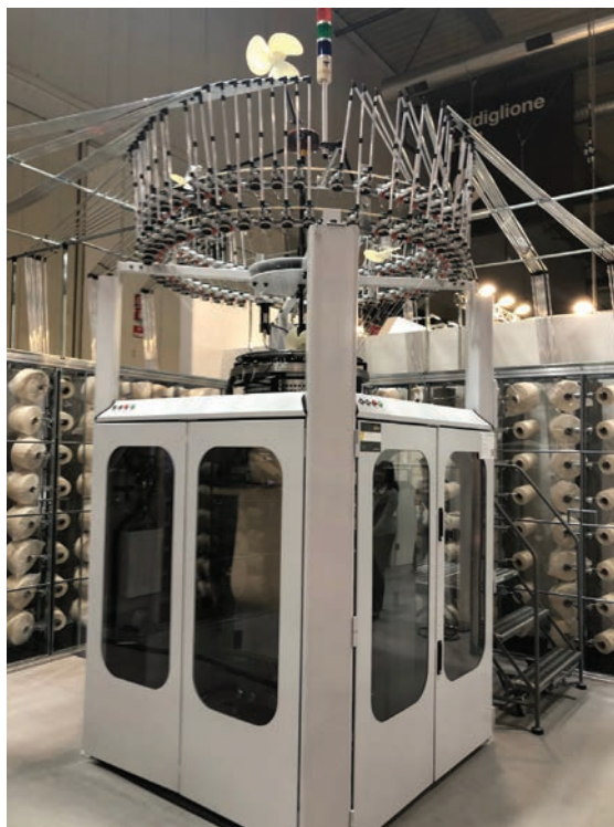
Slika 8: Pletilnik Vanguard Pailung V4SJ1-25CN-I s kvadrastim ogrodjem (vir: https://www.knittingindustry.com/uploads/8454/IMG_3497.jpg )
