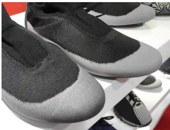
Slika 16: Prstni deli obutve, pleteni s prejo TPU Evolution na pletilniku Colosio S1 (vir: https://districo.com/page-gb/news.html )
