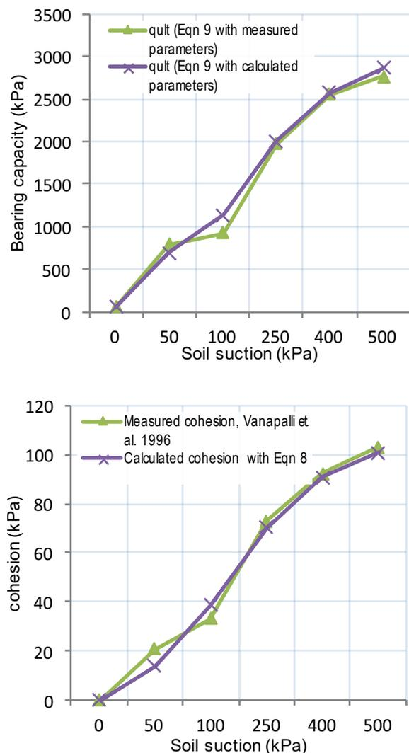
**Figure 2.** Comparison of calculated bearing capacities and total cohesions with measured values.
