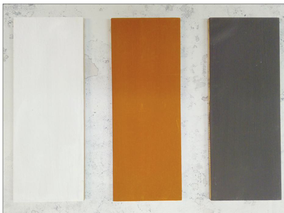
Figure 3. Beech wood samples coated with silicate coatings containing different mineral pigments. From left to right white (titanium dioxide), brown (iron(III) oxide) and deep blue (copper (II) oxide).
