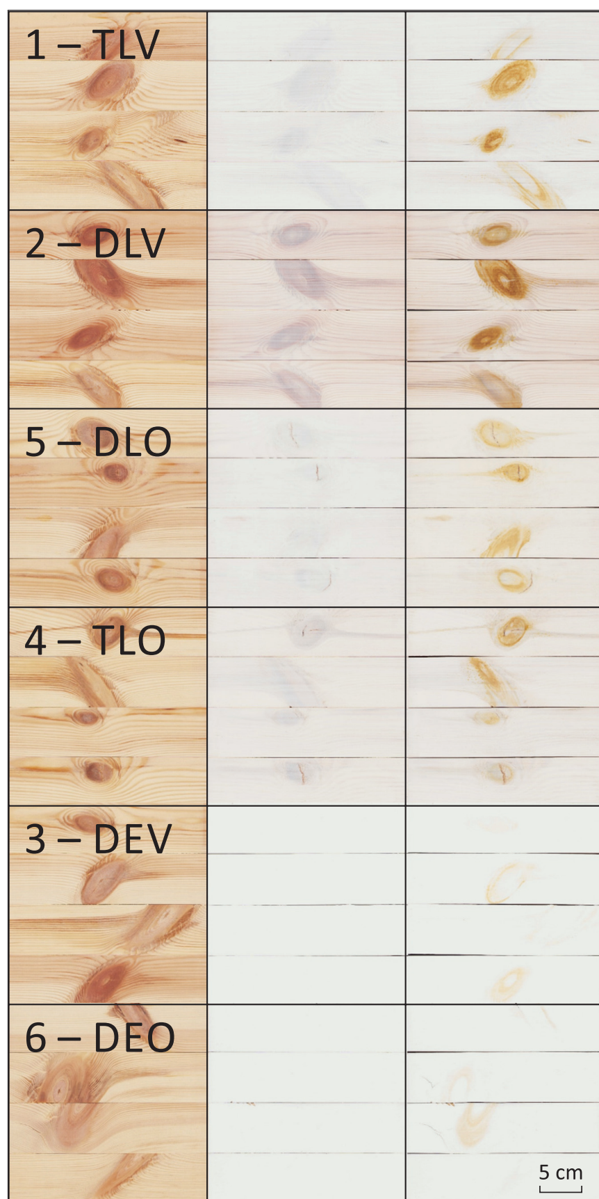
Slika 6. Razvrstitev premaznih sistemov (od 1 do 6) po njihovi odpornosti proti obarvanju (od najslabše zgoraj do najboljše spodaj) glede na barvno razliko pred izpostavitvijo in po njej (levo vzorci pred in v sredini po premazovanju ter desno po UV obsevanju). Figure 6. Classification of coating systems (from 1 to 6) according to their resistance (from the worst to the best) according to the colour difference before and after exposure (left samples before and in the middle after coating and right after UV light exposure).
