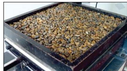
Figure 4. PUR mixed crushed stones.
