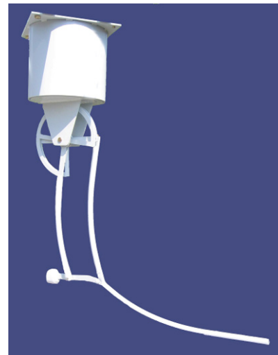
Fig. 3. Manufactured aluminium mechanism used for kinematic tests
