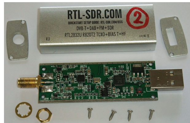
Figure 20: Inexpensive SDR front-end.
