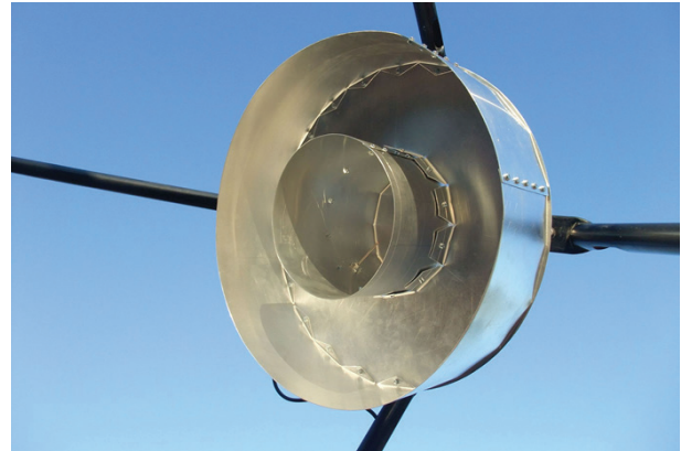
Figure 4: Practical implementation of the VE4MA feed.
