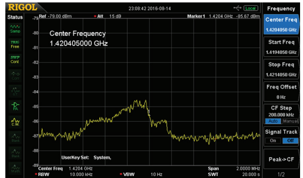
Figure 18: Neutral-hydrogen spectrum from the direction of the star \alpha Scutum.
