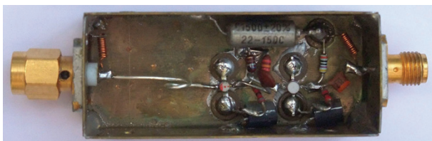
Figure 8: Practical implementation of the LNA.
