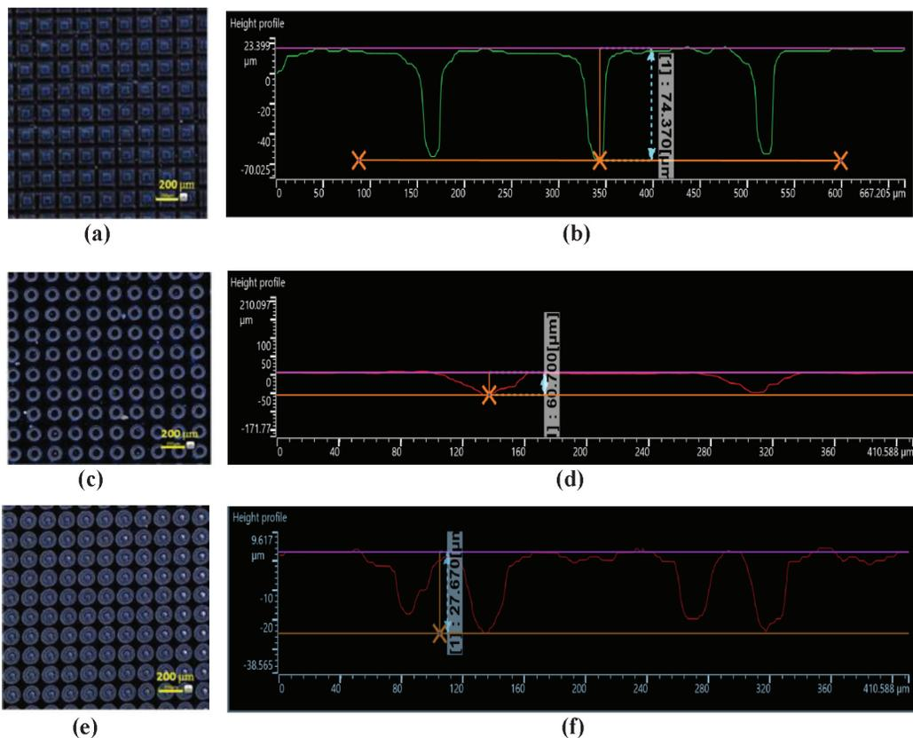
**Figure 1:** Topography of femtosecond-laser-textured surfaces: a) square pillars, b) height profile of square pillars, c) micro-dimples, d) height profile of micro-dimples, e) circumferential grooves, f) height profile of circumferential grooves.
