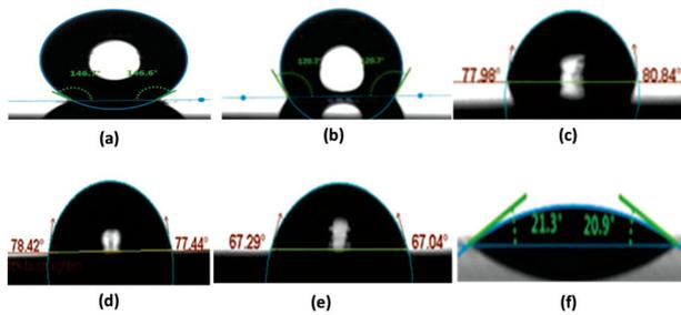
**Figure 3:** Contact angles of textured silicon surfaces: a) Square pillar at laser power 12 W, 60 repetitions, pitch 160 μm, b) Micro dimple at laser power 12 W, 60 repetitions, pitch 160 μm, c) Circumferential groove at laser power 10 W, 60 repetitions, pitch 160 μm, d) Micro dimples at 8 W, 40 repetitions, pitch 190 μm e) Square pillar at 10 W, 60 repetitions, pitch 190 μm f) Circumferential groove at laser power 8 W, 40 repetitions, pitch 220 μm
