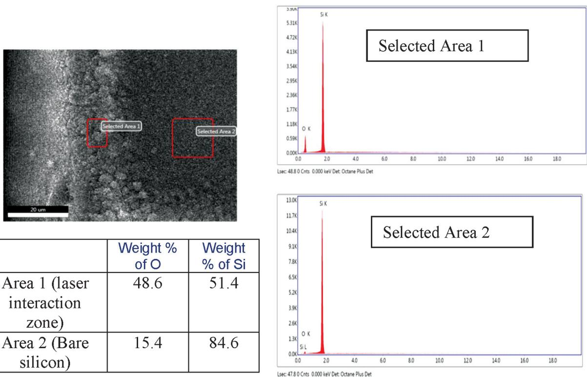
**Figure 7:** XPS Spectra indicating the chemical composition of the laser interacted zone and the non-interacted zone for square pillar texture at laser power 12 W, 60 repetitions, and pitch 160 μm
