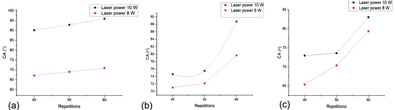
**Figure 5:** Influence of laser power and repetitions on the contact angle: a) square pillar at pitch 190 μm, b) micro dimples at pitch 190 μm, c) circumferential groove at pitch 190 μm
