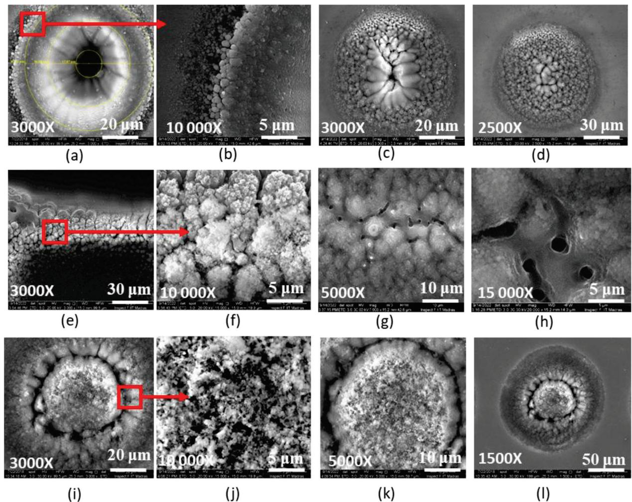
**Figure 2:** SEM Images of laser-treated surfaces: a) micro dimple at 12 W, b) outer layer of the micro dimple at 12 W, c) micro dimple at 10 W, d) micro dimple at 8 W, e) square Pillar at 12 W, f) outer layer of the square pillar at 12 W, g) Square pillar at 10 W, h) square pillar at 8 W, i) circumferential groove at 12 W, j) outer layer of circumferential groove at 12 W, k) circumferential groove at 10 W, l) circumferential groove at 8 W
