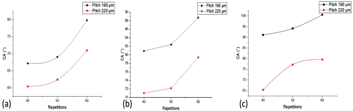
**Figure 6:** Influence of pitch and repetitions on the contact angle: a) square pillar at laser power 8 W, b) micro-dimples at laser power 8 W, c) circumferential grooves at laser power 8 W
