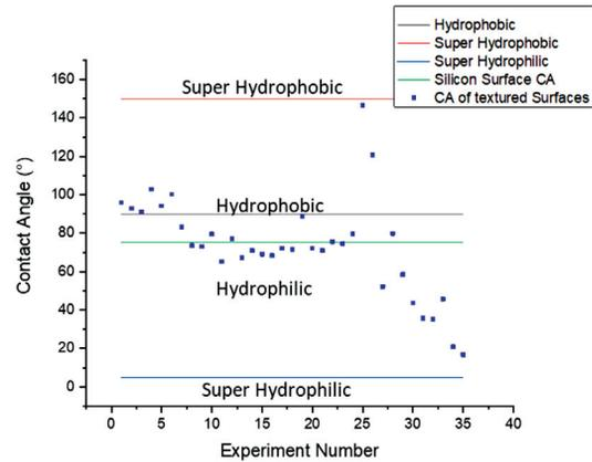
**Figure 4:** Spectrum of contact angles for the textured N-Type silicon surfaces
