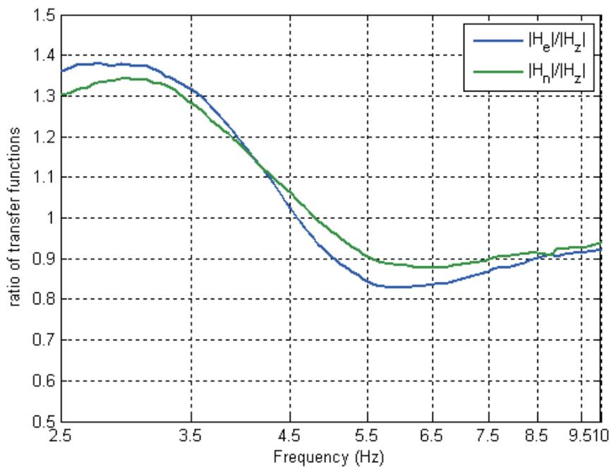
**Figure 7.** The ratio of the transfer functions of the TROMINO TR-19 seismological system computed using equation (26): the ratio of the transfer function of the E-W component and the vertical component (blue line) and the ratio of transfer function of the N-S component and the vertical component (green line). Below 3 Hz, the self-noise of the Tromino TR-19 affects the calculation and below this frequency, the ratio of the transfer functions cannot be calculated in this particular case.
