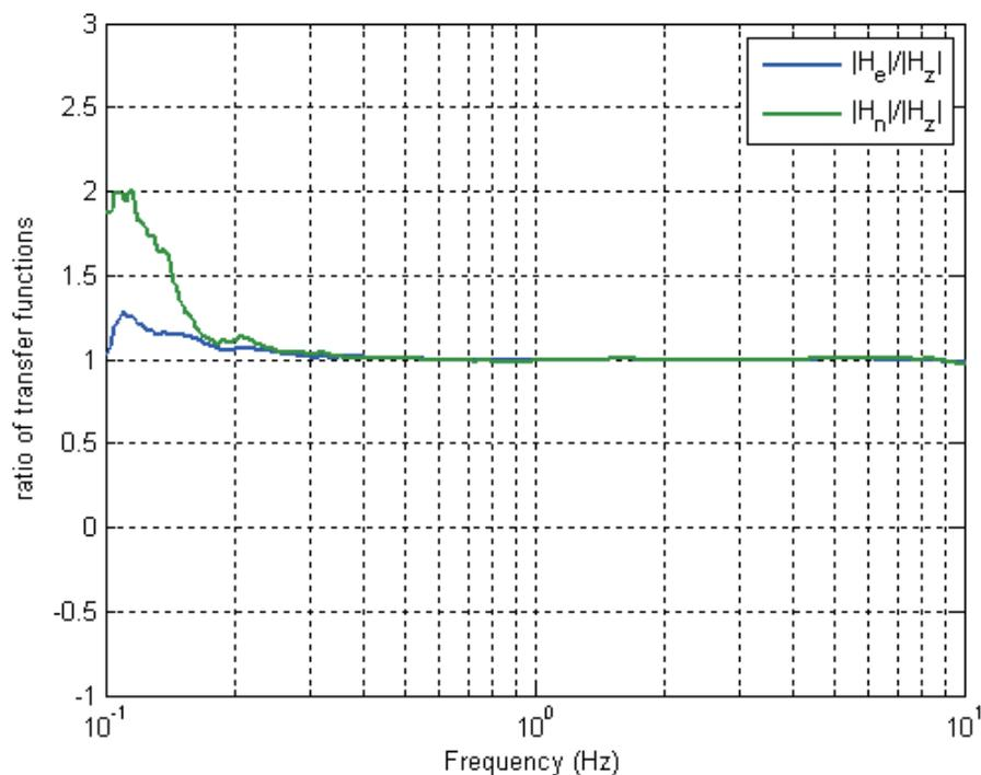
**Figure 5.** The ratio of transfer functions for an LE-3D/5s seismological system computed using equation (26), the ratio of the transfer functions of the E-W and the vertical component (blue line), the ratio of the transfer function of the N-S component and the vertical component (green line). The ratio of the transfer functions drastically changes its slope at 0.11 Hz and can be explained by the influence of the instrumental noise.
