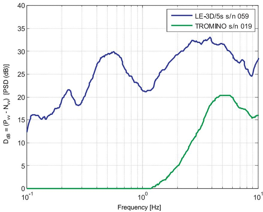
**Figure 6.** The difference between the PSD of the estimated self-noise curve ( $N_{vv}$ ) estimated by “Three-channel Correlation Analysis Techniques” [19] and the PSD of the recorded seismic signal ( $P_{vv}$ ) for the LE-3D/5s seismometer (s/n 59) and TROMINO (TR 19), for the vertical component. The self-noise of the TROMINO instrument is considerably higher.
