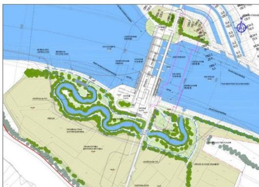
Fish Pass 1, on the right bank, is 655 m long, and has an average longitudinal gradient of 1.3%, the total length of 6 spawning grounds in the close-to-nature section is 180 m, and all spawning grounds are the same length and more than 9 m wide. The spawning grounds are designed in the form of two parallel corridors, so that the spawning of lithophilic spawners is enabled along one bank, while along the other bank fish can pass upstream in all sections.
