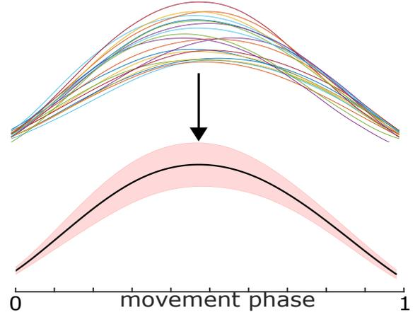
Figure 3: Trajectory distribution model calculated from several different trajectories. This model represents only one degree of freedom.
