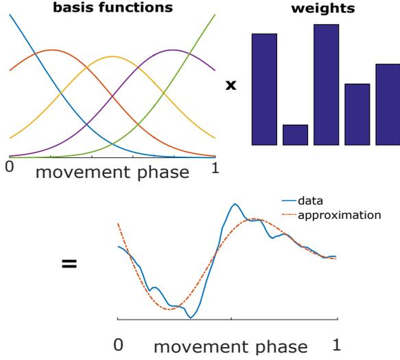
Figure 2: Approximating a sequence of states using 5 basis functions and their corresponding weights.
