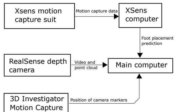
Figure 1: Block diagram of the setup used in the experiment.
