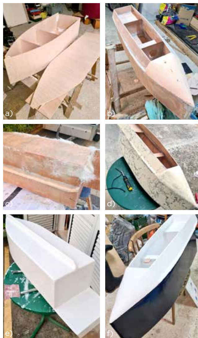
Figure 2 : Stages of boat hull construction, a) screw connection, b) polyester binding, c) plasticizing, d) coating with cement kit, e) primer coating, f) coating with final paint
